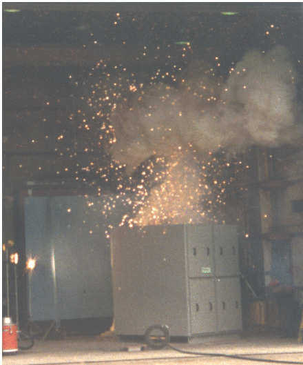
Figure 3. Successful arc test on 15 kV metal-clad switchgear.
