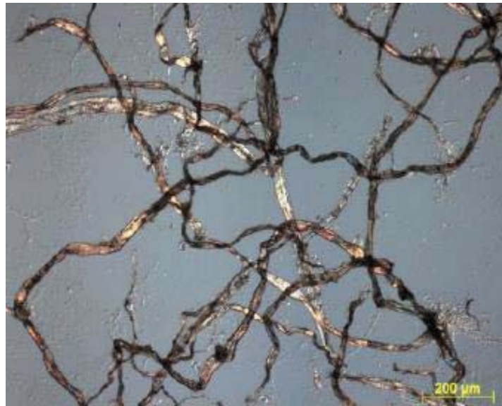
Figure 3: Kraft fibres treated to induce curl (source, FPInnovations)
