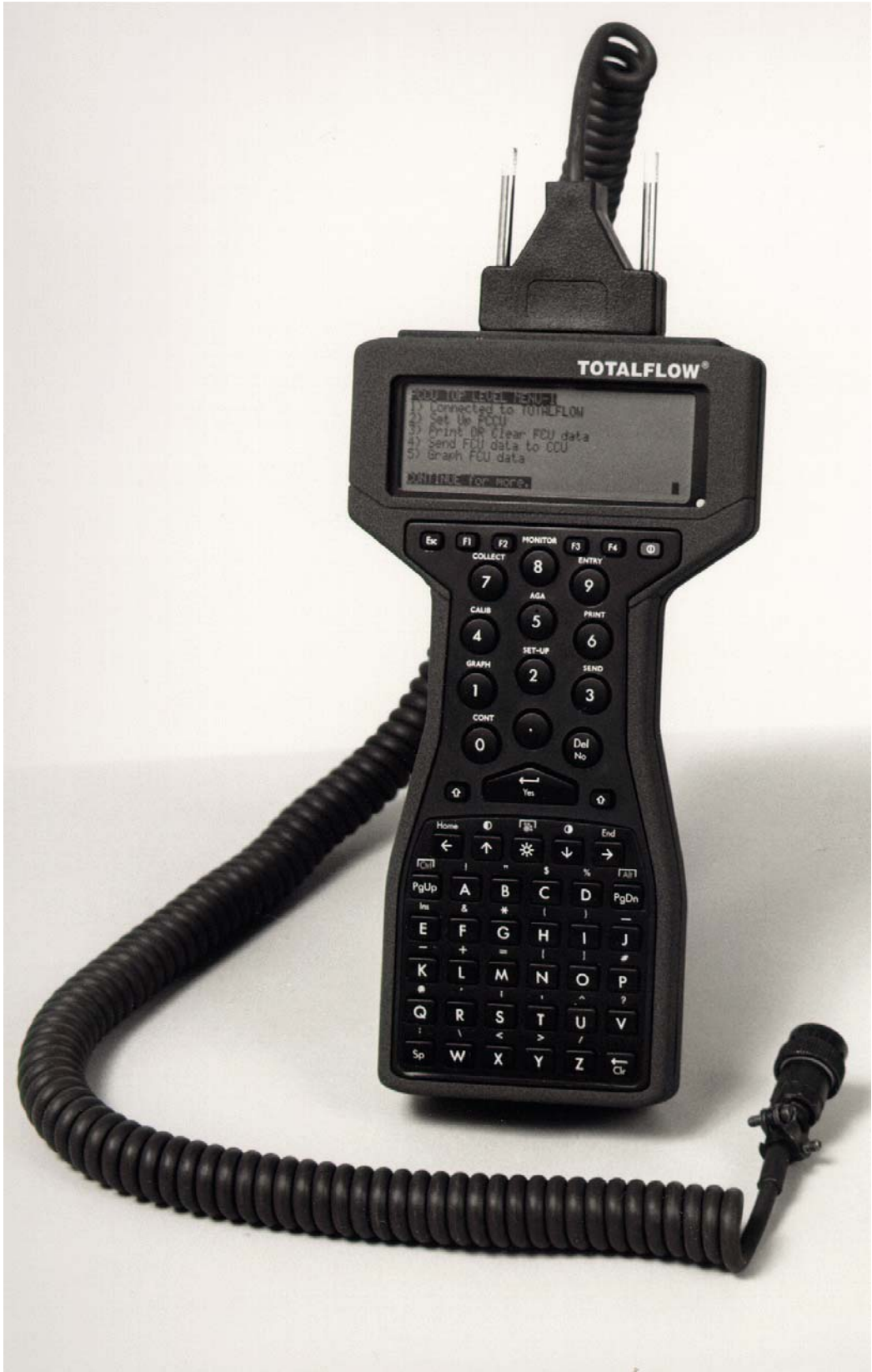
Figure 3-1 Totalflow Portable Calibration & Collection Unit (PCCU)
