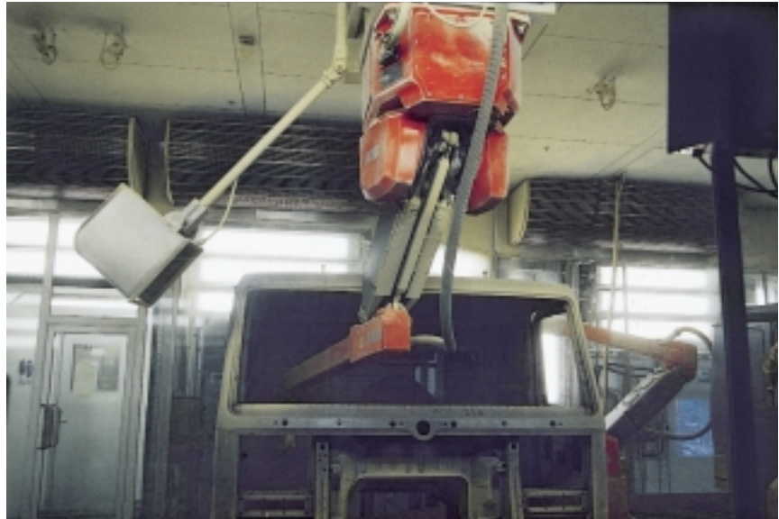
Powder is applied to the inside and outside of the cab roof by a robot, equipped with a dual gun, attached to the ceiling of the booth. 4
