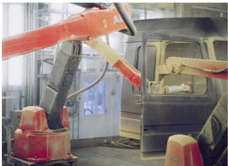
A robot mounted on a conveyor paints the inside and edges of the doors as well as a section of the inside wall of the cab. The doors are opened and closed by another robot (on right). 5
