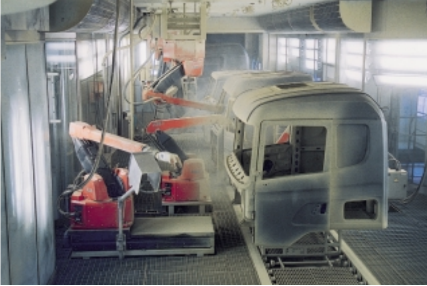
The robot used to apply the powder coating to the inside of the cab is mounted on a conveyor and equipped with a dual gun. It reaches through the windshield opening and applies the powder to the rear and side inner walls; the rear part of the floor can also be painted if necessary.
