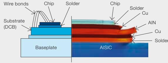
Cross-section schematic of IGBT module. Right: FE simulation showing deformation caused by thermal cycling (100 x saturated). [Source: Samuel Hartmann]
