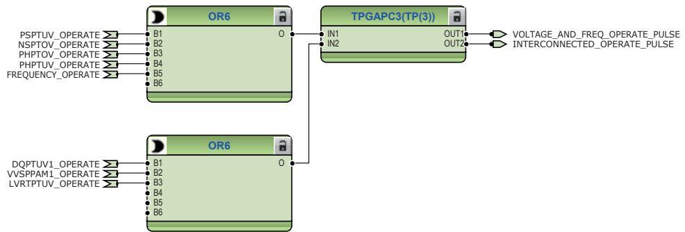
Figure 72: Timer logic for voltage/frequency and interconnected protection operate pulse
