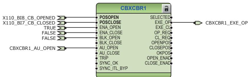
*Figure 110: Circuit breaker 1 control logic*
