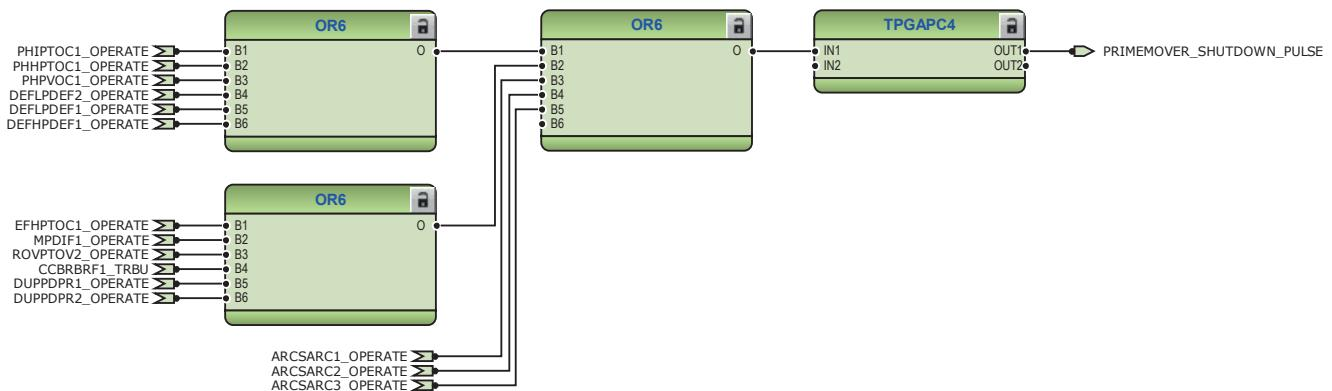
Figure 190: Timer logic for primemover shutdown pulse
