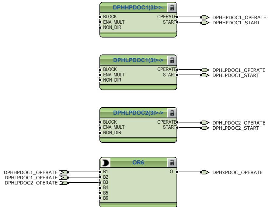
*Figure 16: Directional overcurrent protection function*
