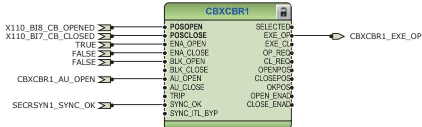
Figure 168: Circuit breaker 1 control logic
