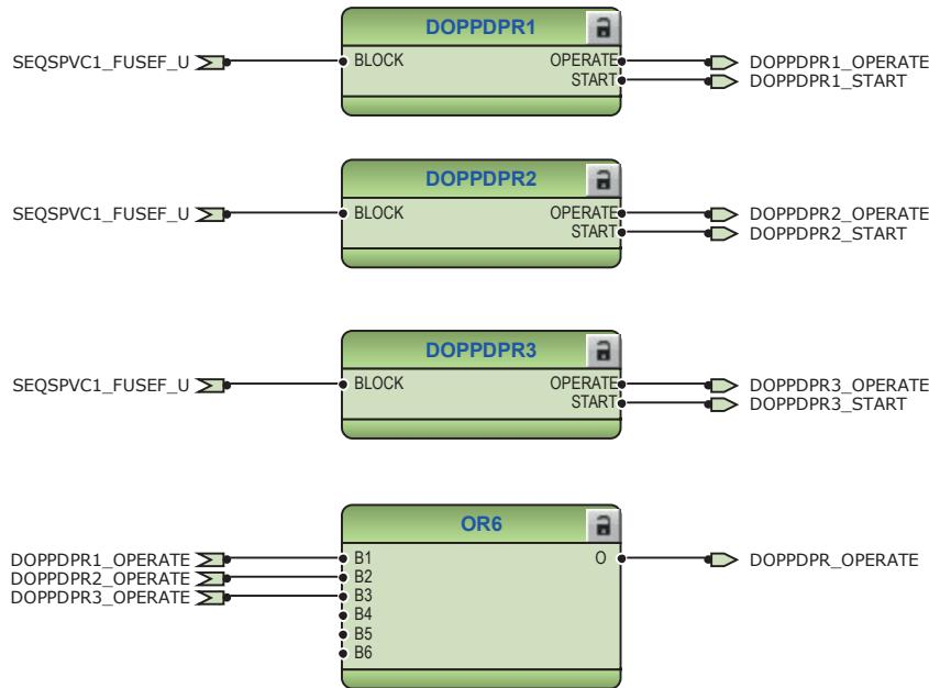
*Figure 91: Directional overpower protection function*
