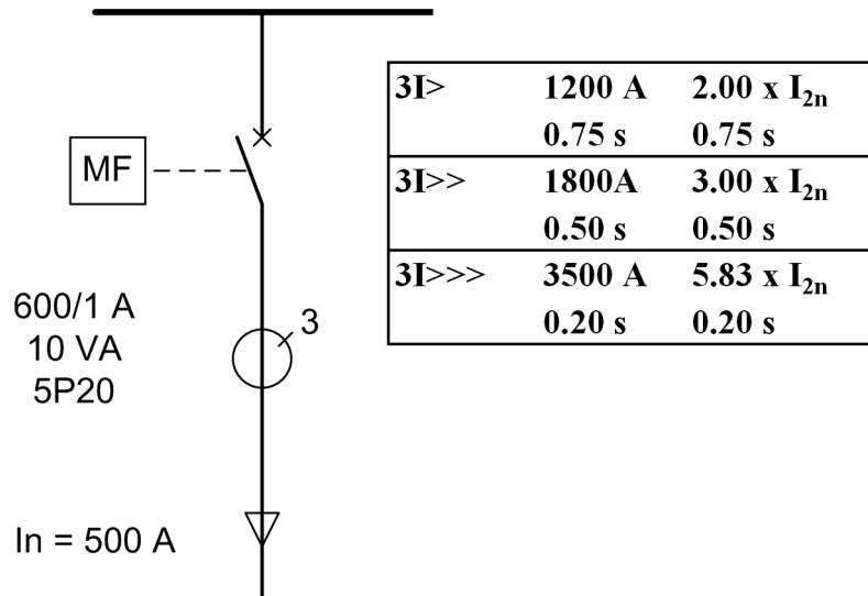
Figure 193: Example of three-stage overcurrent protection
