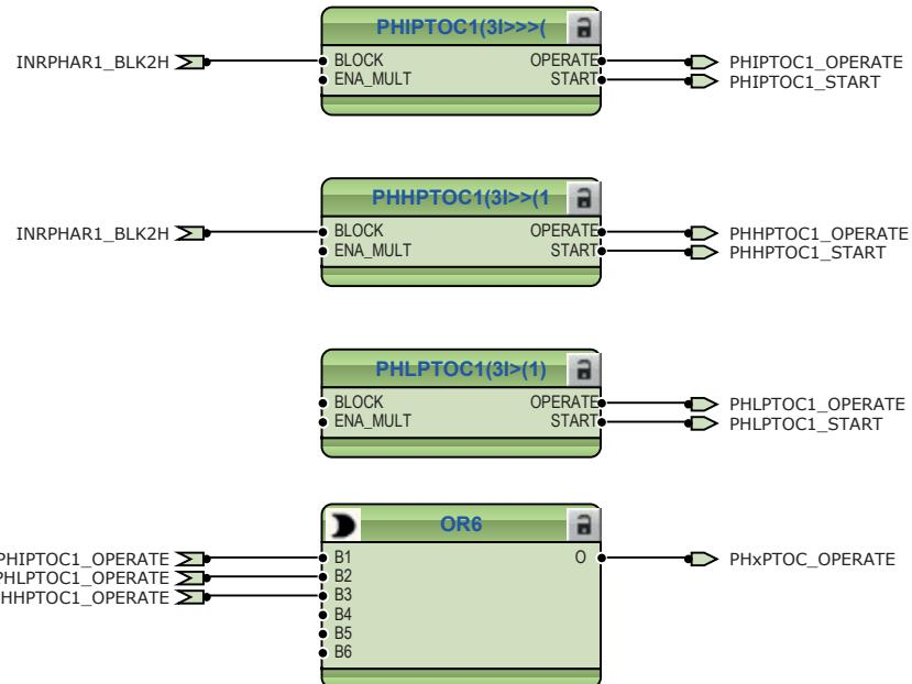
*Figure 74:* Overcurrent protection function
