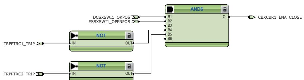
Figure 51: Circuit breaker 1 close enable logic
