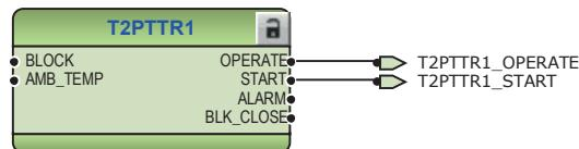
Figure 143: Thermal overcurrent protection function
