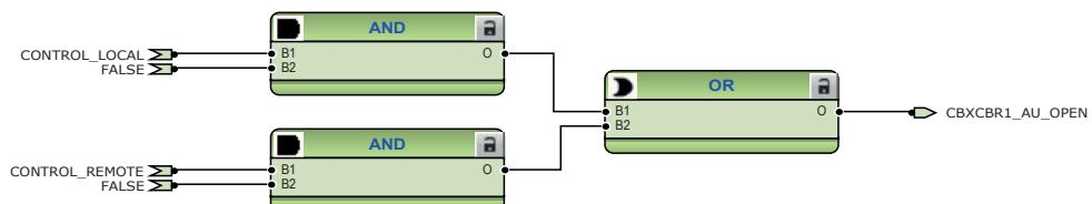
Figure 54: External opening command for circuit breaker 1
