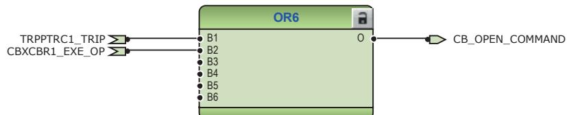
*Figure 111: Signal for opening coil of circuit breaker 1*
