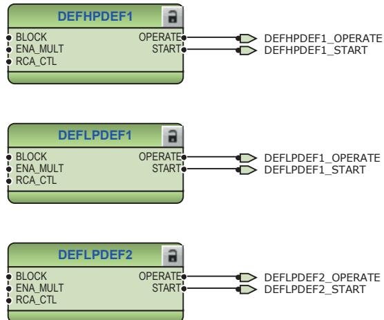
Figure 78: Directional earth-fault protection function
