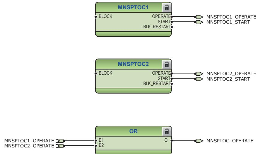
Figure 77: Negative sequence overcurrent protection function
