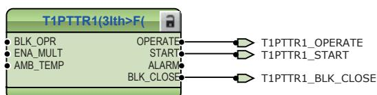
*Figure 20: Thermal overcurrent protection function*
