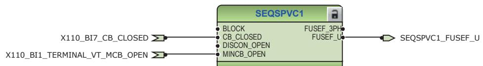
Figure 159: Fuse failure supervision function
