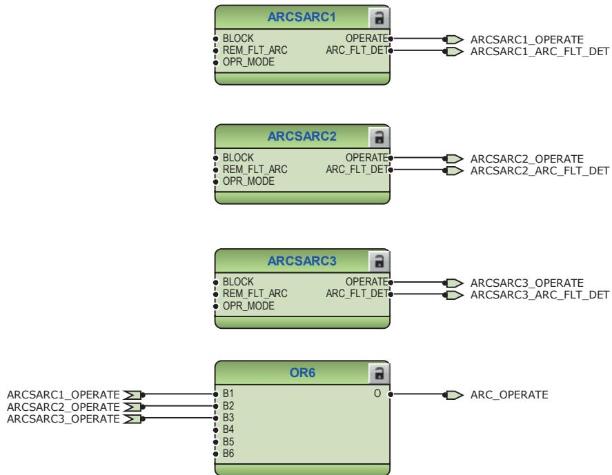
Figure 83: Arc protection function
