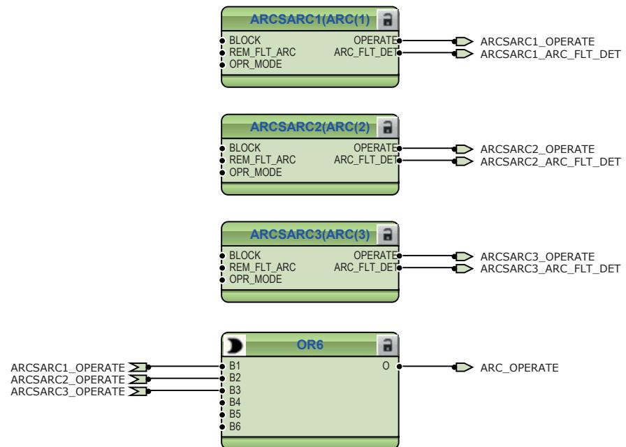
Figure 22: Arc protection function
