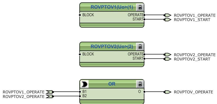
*Figure 26:* Residual overvoltage protection function
