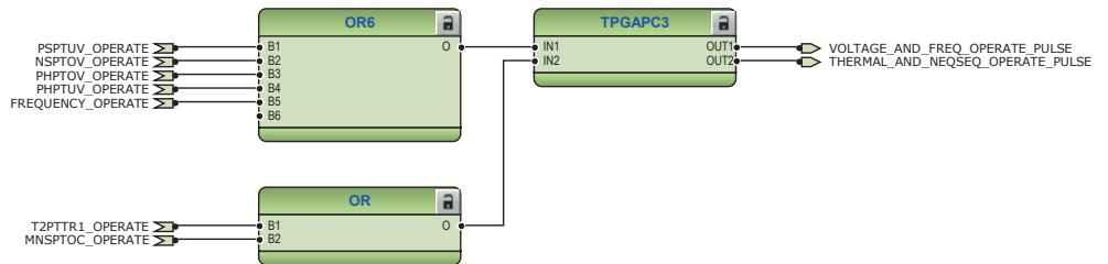
*Figure 131: Timer logic for voltage/frequency and interconnected protection operate pulse*
