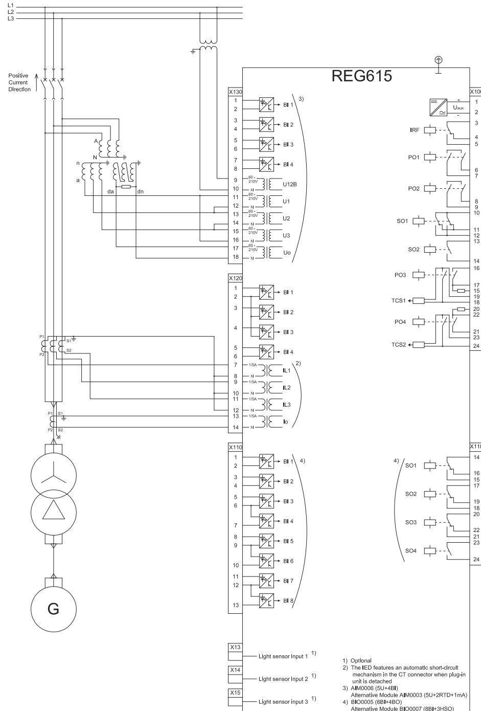
Figure 11: Connection diagram for the A configuration
