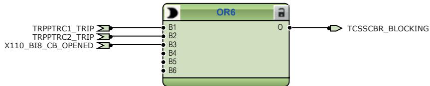
Figure 44: Logic for blocking of trip circuit supervision
