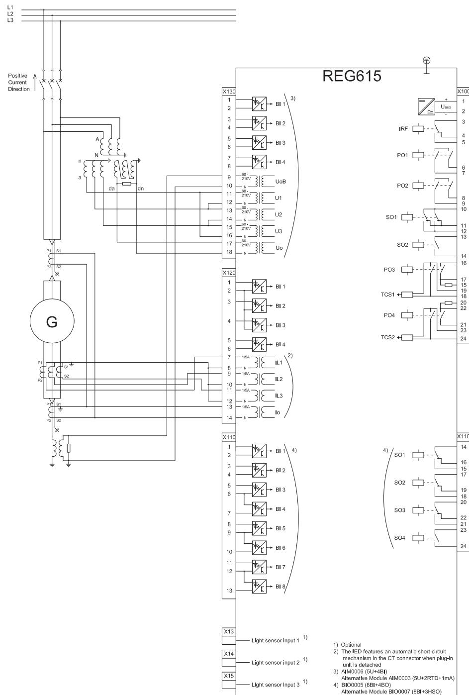
Figure 12: Connection diagram for the C configuration
