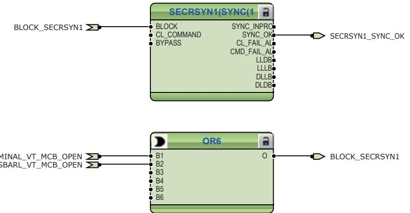
*Figure 45: Synchrocheck function*
