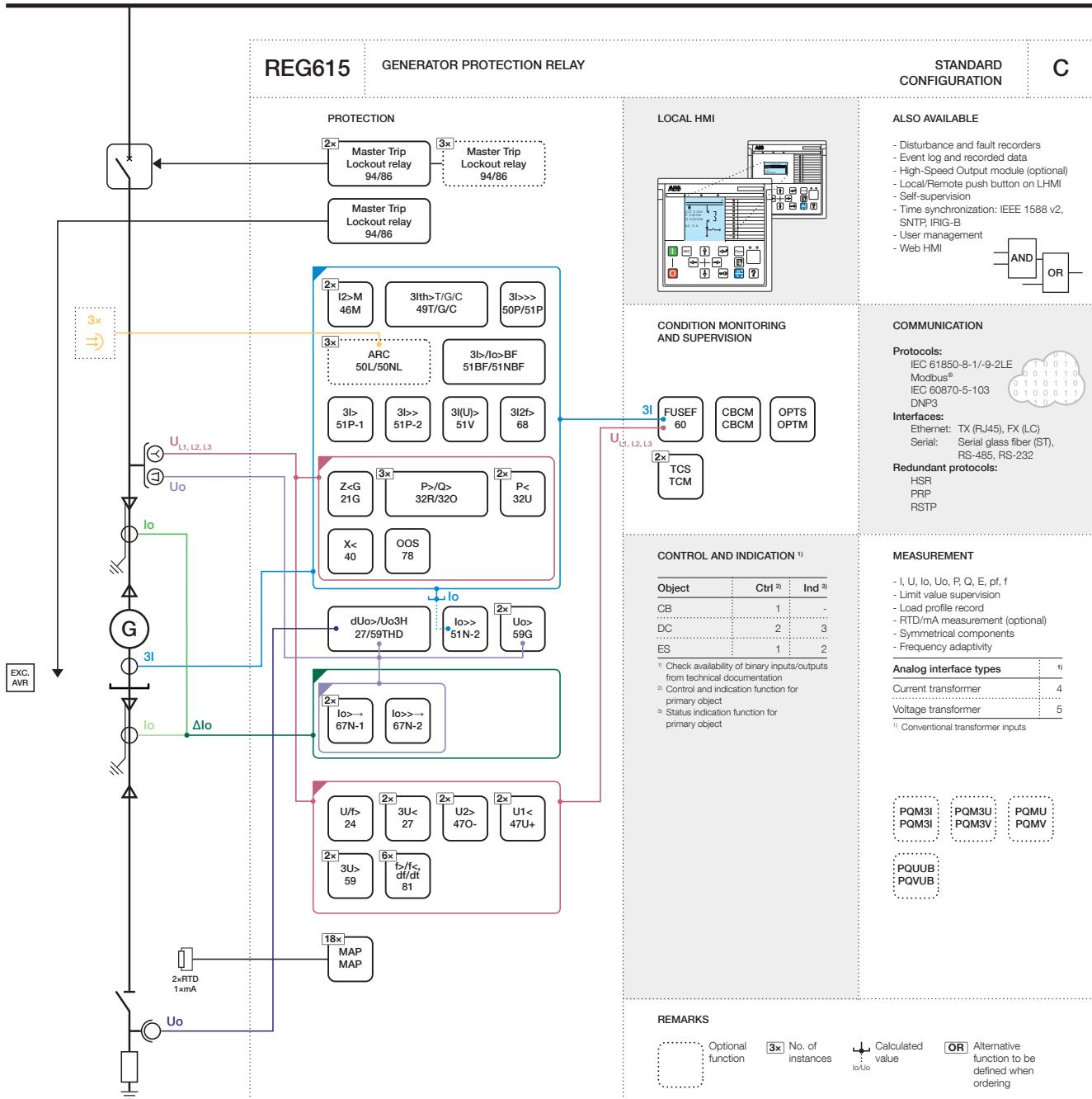
Figure 73: Functionality overview for standard configuration C
