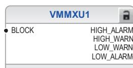
Figure 58: Voltage measurement: Three-phase voltage measurement (Terminal side)
