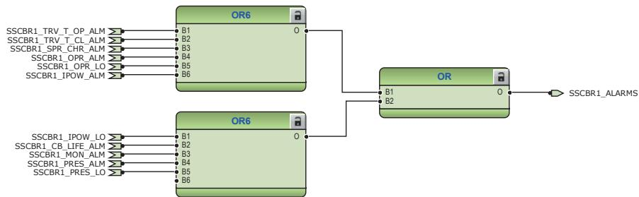
Figure 103: Logic for circuit breaker monitoring alarm
