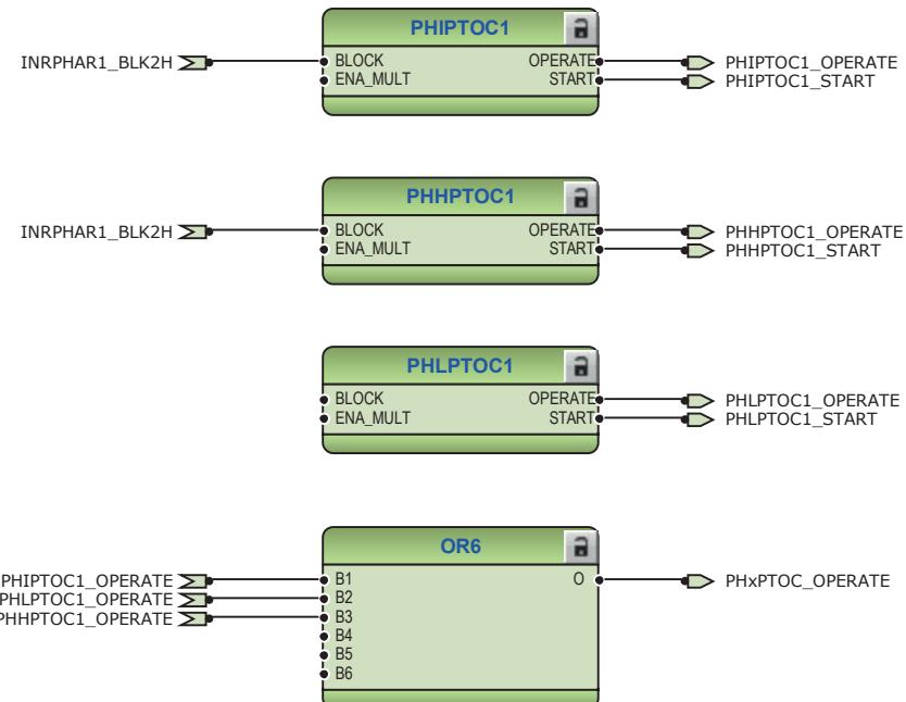
Figure 137: Non directional overcurrent protection function
