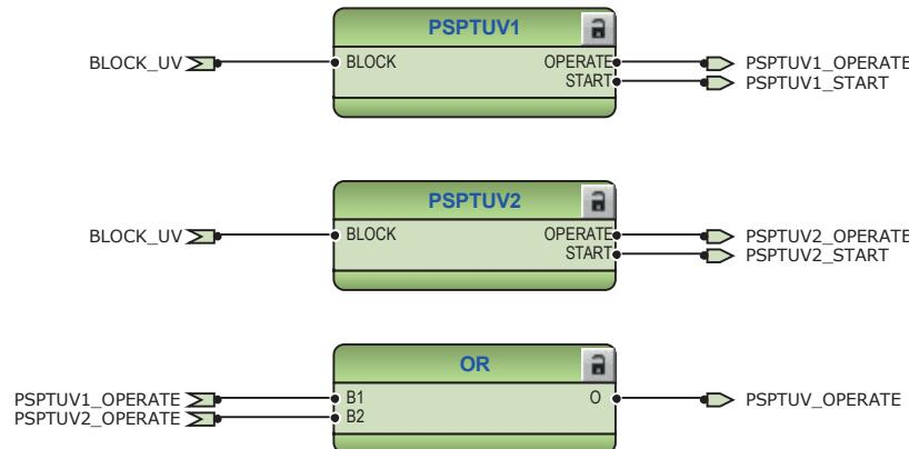
*Figure 88: Positive sequence undervoltage protection function*
