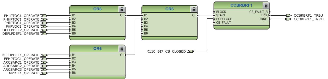
*Figure 145: Circuit breaker failure protection function*
