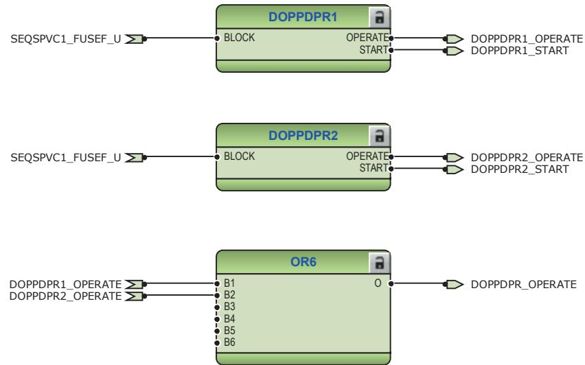
Figure 150: Directional overpower protection function
