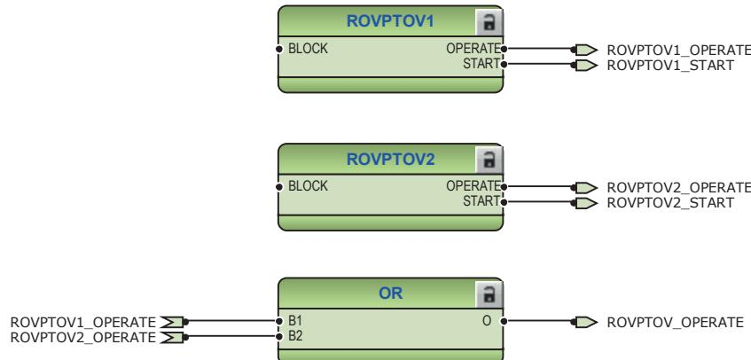
*Figure 89: Residual overvoltage protection function*
