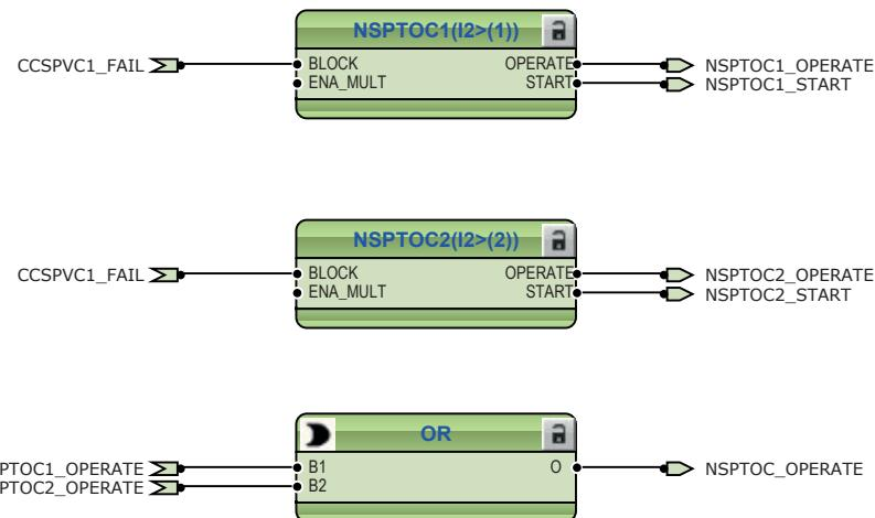
*Figure 18: Negative sequence overcurrent protection function*
