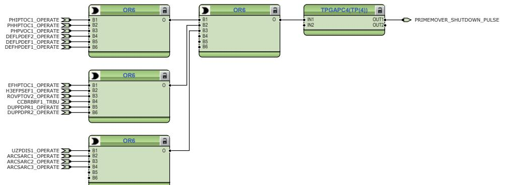
*Figure 132: Timer logic for primemover shutdown pulse*
