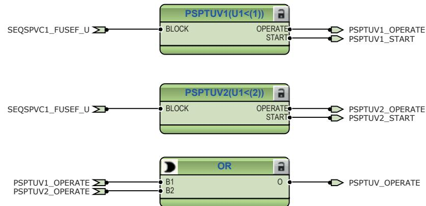
Figure 28: Positive sequence undervoltage protection function
