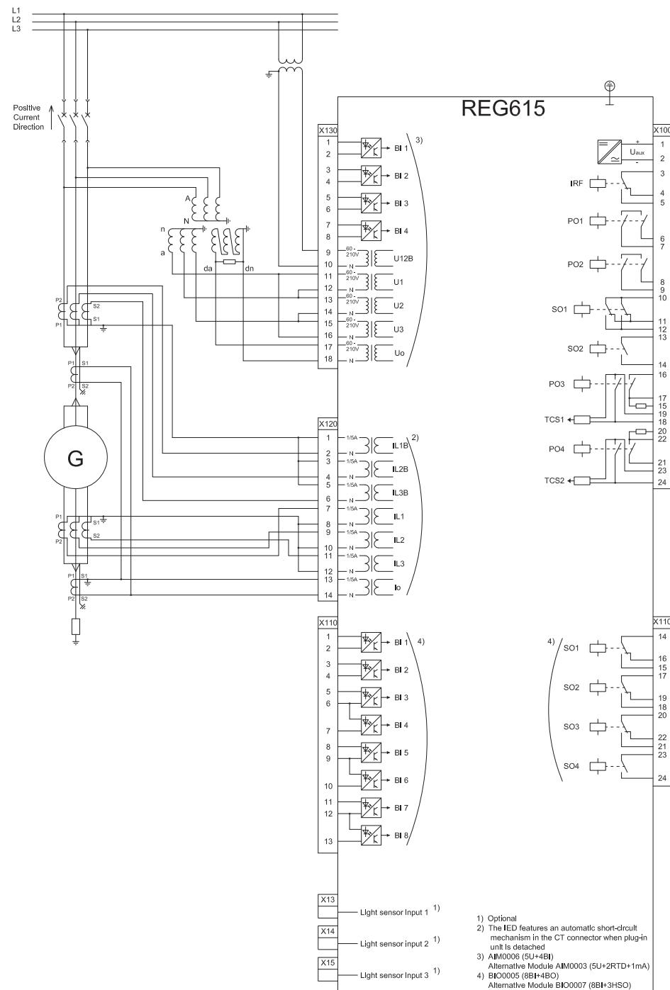
Figure 13: Connection diagram for the D configuration
