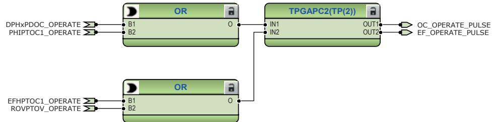
Figure 71: Timer logic for overcurrent and earth-fault operate pulse
