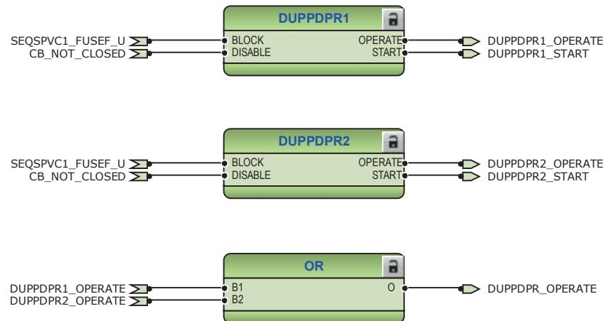
Figure 151: Directional underpower protection function
