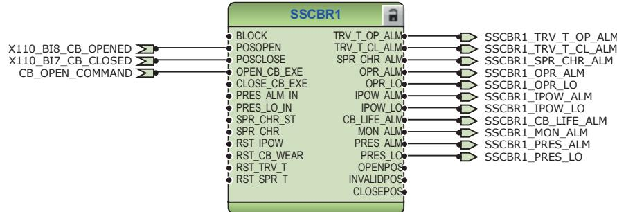
*Figure 160: Circuit breaker condition monitoring function*
