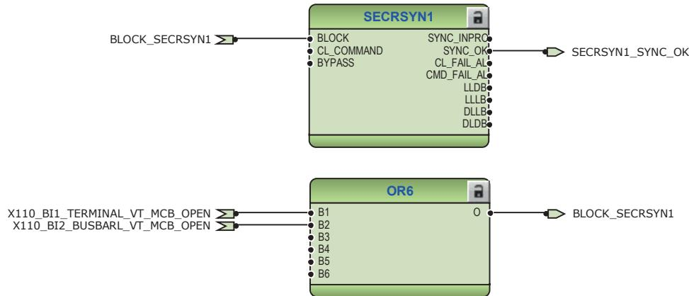
*Figure 165: Synchrocheck function*
