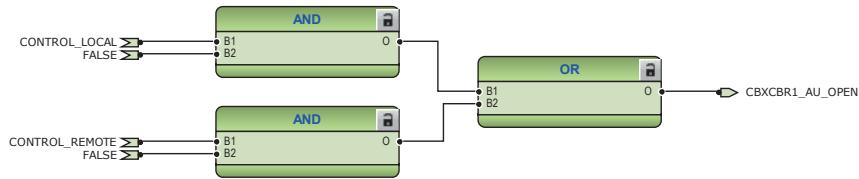
Figure 112: External opening command for circuit breaker 1
