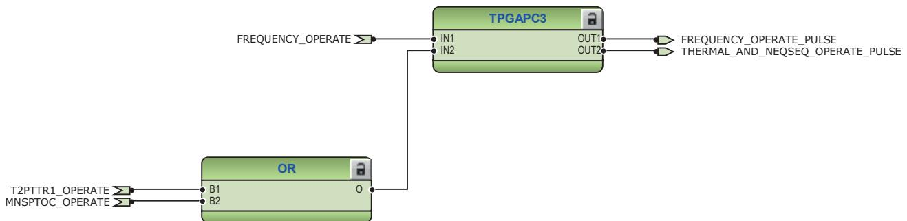
Figure 189: Timer logic for voltage/frequency and thermal/negative sequence protection operate pulse
