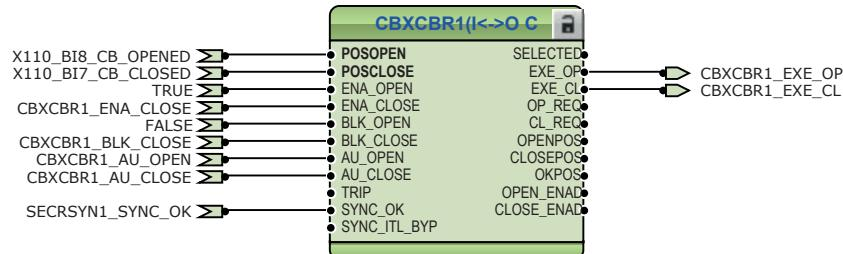
Figure 48: Circuit breaker 1 control logic
