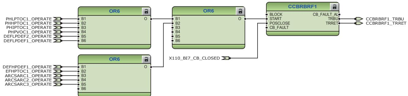
Figure 82: Circuit breaker failure protection function
