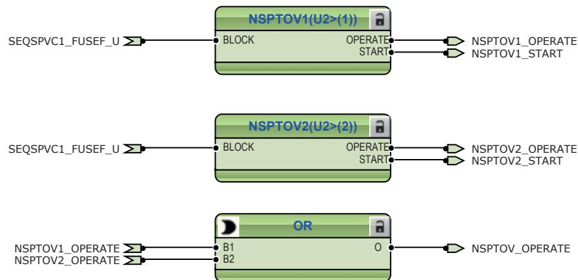
Figure 27: Negative sequence overvoltage protection function
