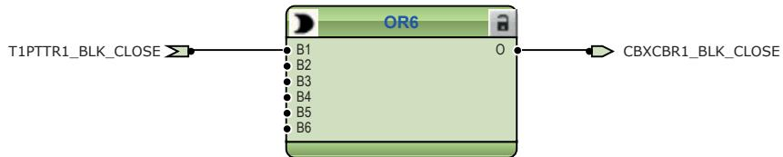
Figure 52: Circuit breaker 1 close blocking logic
