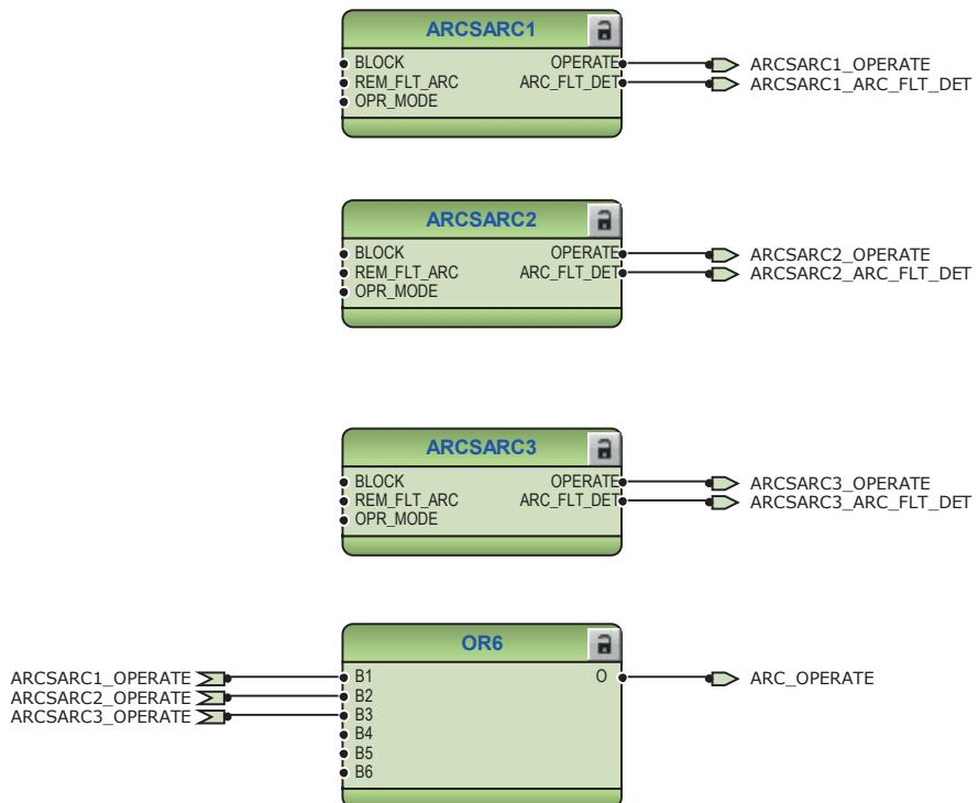
*Figure 146: Arc protection function*
