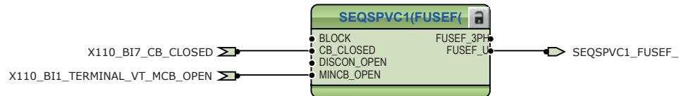
*Figure 39: Fuse failure supervision function*
