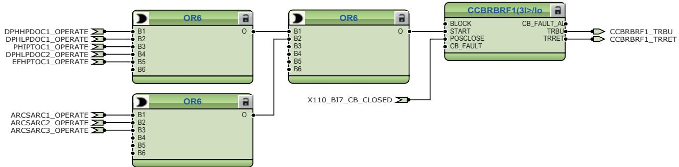
*Figure 21: Circuit breaker failure protection function*
