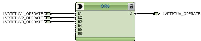
Figure 33: Low voltage ride through protection function
