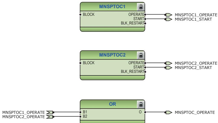
*Figure 140: Negative sequence overcurrent protection function*
