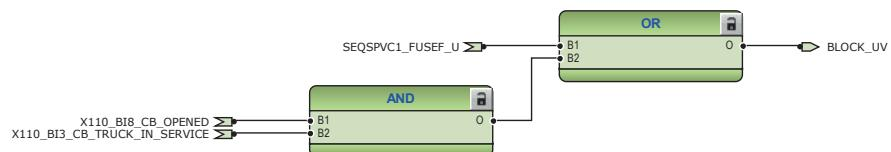
*Figure 133: Blocking logic for undervoltage protection*
