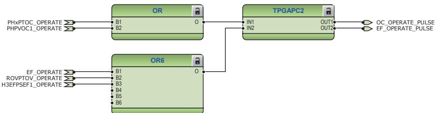
*Figure 130: Timer logic for overcurrent and earth-fault operate pulse*
