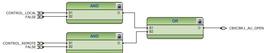
Figure 170: External opening command for circuit breaker 1
