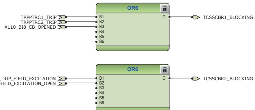
Figure 163: Logic for blocking of trip circuit supervision
