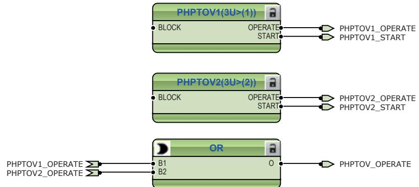
*Figure 24:* Overvoltage protection function
