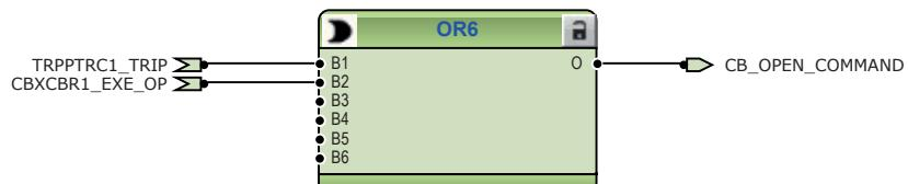
Figure 50: Signal for opening coil of circuit breaker 1
