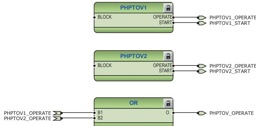
*Figure 85:* Overvoltage protection function
