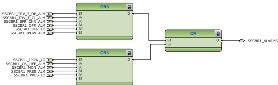
*Figure 161: Logic for circuit breaker monitoring alarm*
