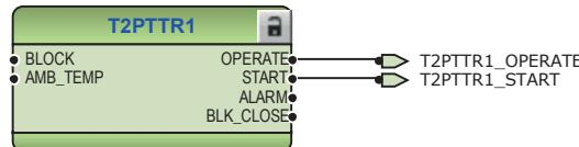
*Figure 81: Thermal overcurrent protection function*
