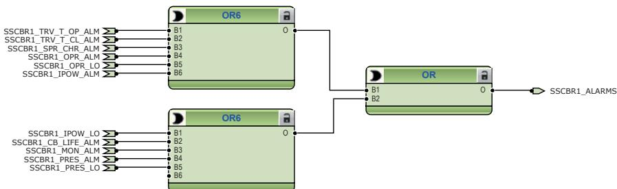
*Figure 41: Logic for circuit breaker monitoring alarm*
