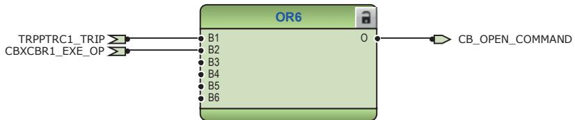
Figure 169: Signal for opening coil of circuit breaker 1
