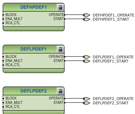
*Figure 141: Directional earth-fault protection function*
