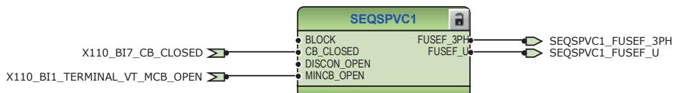
Figure 101: Fuse failure supervision function
