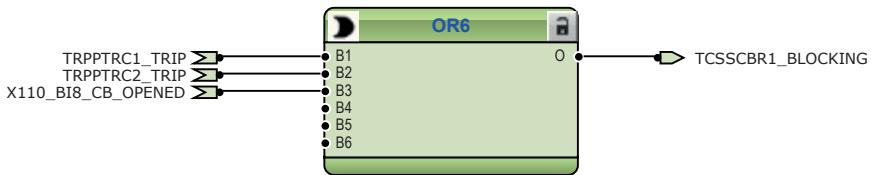
Figure 106: Logic for blocking of trip circuit supervision
