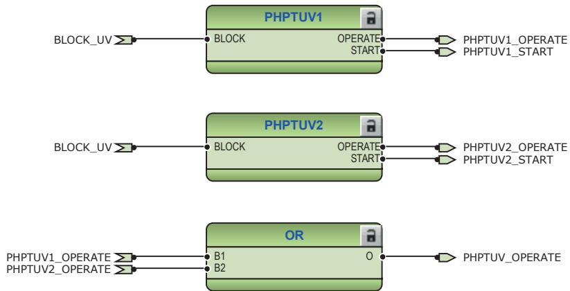
Figure 86: Undervoltage protection function
