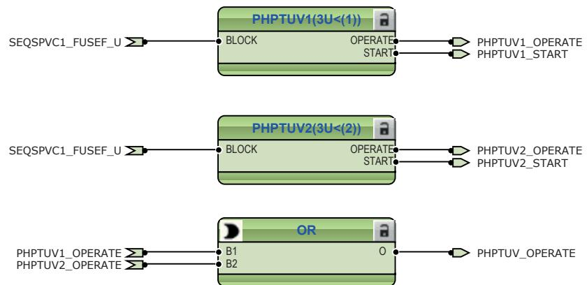
*Figure 25:* Undervoltage protection function
