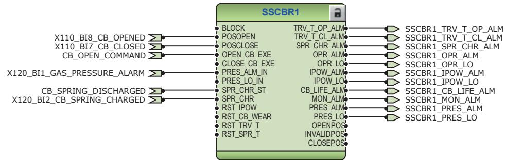
Figure 102: Circuit breaker condition monitoring function
