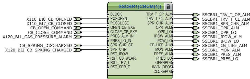
*Figure 40: Circuit breaker condition monitoring function*
