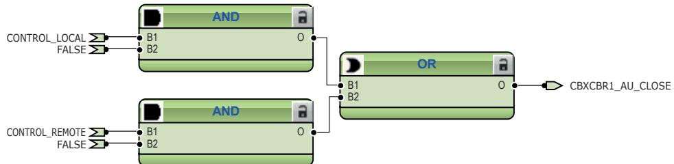
Figure 53: External closing command for circuit breaker 1
