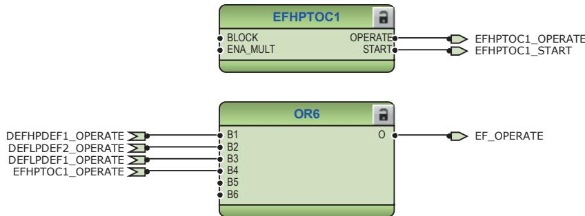
*Figure 79: Earth-fault protection function*
