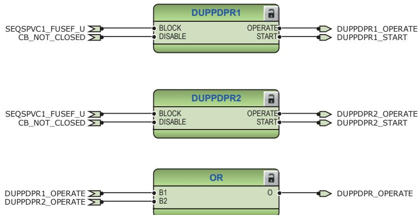
*Figure 92: Directional underpower protection function*
