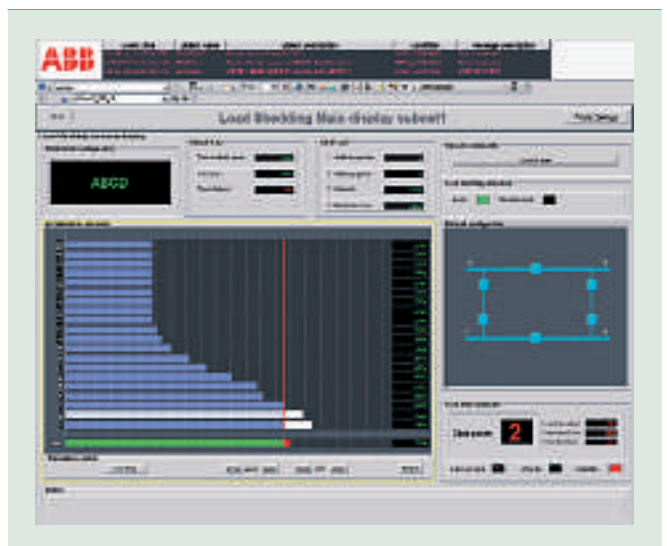
4 Graphical presentation of the accumulated effect of shedding the loads assigned to the 20 load shedding priorities.
