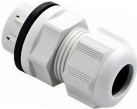
ABB's latest cable gland offering, the NPG Quick-Connect™, allows for fast and effective fitting without access to the inside of an enclosure, greatly speeding installation. The speed and ease of installation makes the NPG ideal for panel builders and volume installers of all types. NPG Quick-Connect™ is a single-piece, corrosion resistant nylon gland suitable for non-armoured, portable and tray cable types. When installed, the NPG achieves ingress protection of IP66 or IP68 (5 bar 30 mins).
