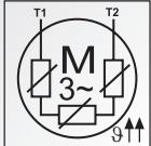
CM-MSE and CM-MSS provide full protection of motors with integrated PTC resistor sensors.
