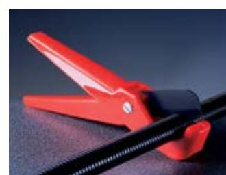
Place the conduit between the cutting blade and lower support, squeeze the handles and rotate the conduit for a clean, easy cut. Spare blades are available.
