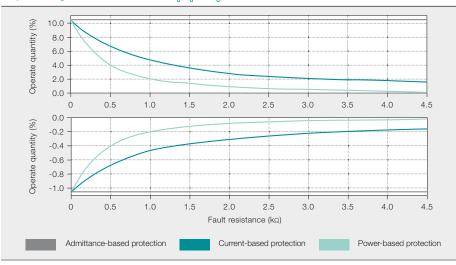
resulting from the compensation effect of the Petersen coil. Often, these currents are only a fraction of the normal load current, too low to trip conventional overcurrent relays.
