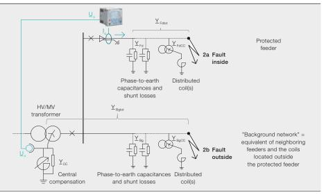
to traditional earth-fault protection, where the magnitude of the operate quantity, based on residual current or power, is greatly decreased by the fault resistance. This feature of the neutral admittance principle improves the sensitivity of the earth-fault protection and enhances discrimination between fault and nonfault conditions, especially at higher fault resistance values  $\rightarrow$  1.
