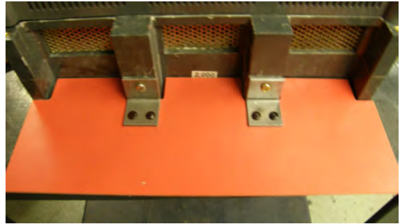
Figure 6: Line Shield Installation
