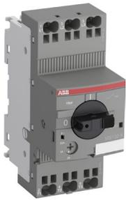
The MS132-K series is a compact and powerful range for motor protection up to 15 kW (400 V) / 32 A with a width of only 45 mm. The innovative Push-in Spring terminals enable tool-free wiring and eliminate the need for routine re-tightening. The manual motor starter is suitable for three- and single phase applications.
