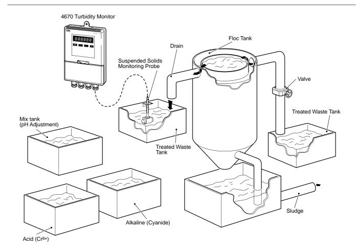
The illustration above shows how process liquers are first treated in the cyanide or chrome tanks (see relevant Application Guides) then mixed in a mix tank where the pH is adjusted to between 8 and 9pH.
