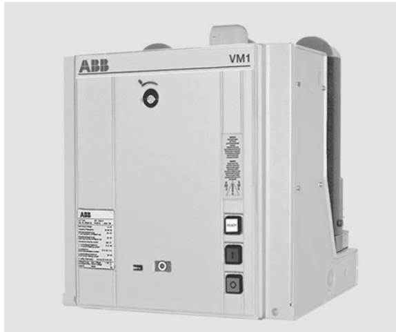
Figure 9/1: Vacuum circuit breaker, type VM1-T, for fixed installation, 12 kV, \leq 1250 A, \leq 25 kA, mechanism side.
