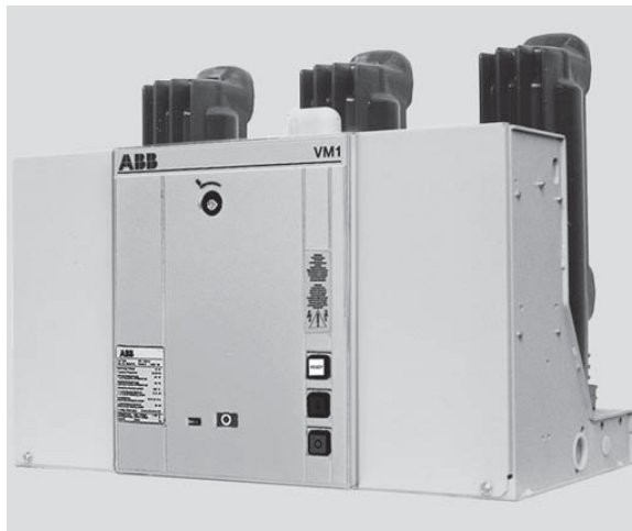
Figure 9/3: Vacuum circuit breaker, Typ VM1-T, for fixed installation, 12 kV, 1600 ... 2000 A, 25 kA, mechanism side.
