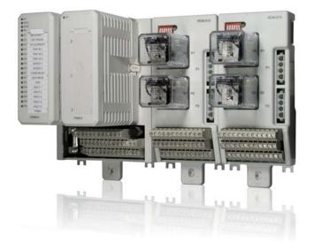
All four turbine specialty modules have embedded processors which execute their specific functions, and while they can exchange data with the main controller over PROFIBUS, they operate independently of it.
