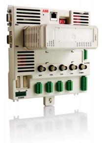
Symphony Plus offers a fully integrated condition monitoring solution comprising MCM800, an 'all-in-one' hardware module that can be easily programmed for all vibration and turbine supervisory functions, and Analyst, a user-driven graphical analysis software that creates specialized plots for use in assessing the condition of rotating machinery.
