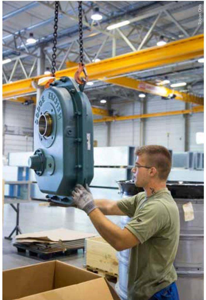
By partnering with ABB, the GSI Hungary facility was able to locally source their preferred Dodge brand of mechanical power transmission products, including this Torque-Arm II shaft mount gear reducer.
