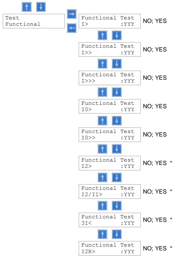
Figure 25: Functional test menu of relay REF601/REJ601/REM601
