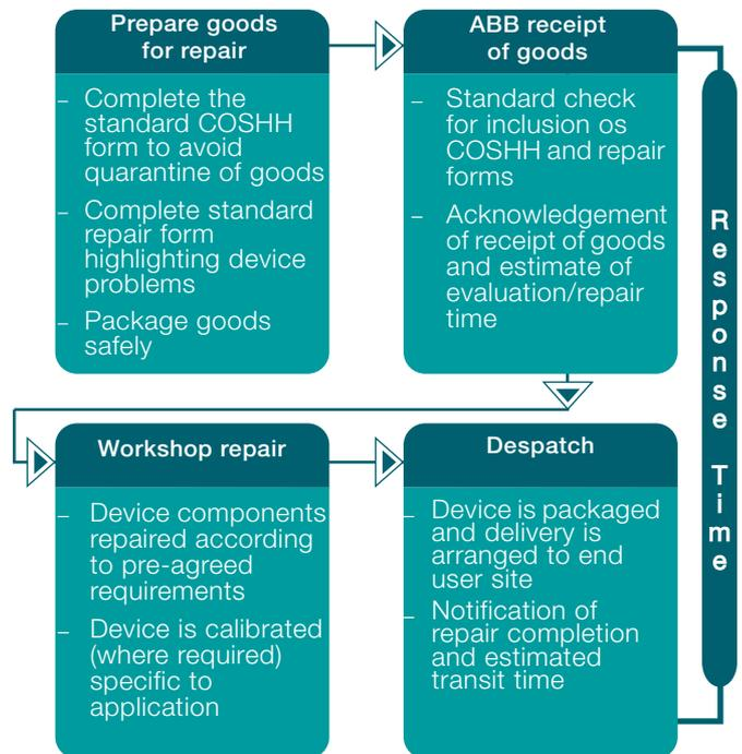
Fig. 3: ABB workshop repairs process
