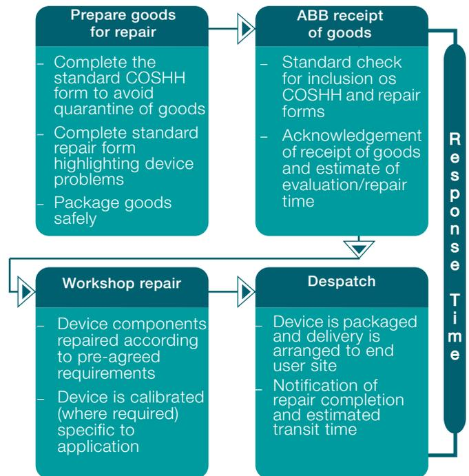
Fig. 3: ABB workshop repairs process
