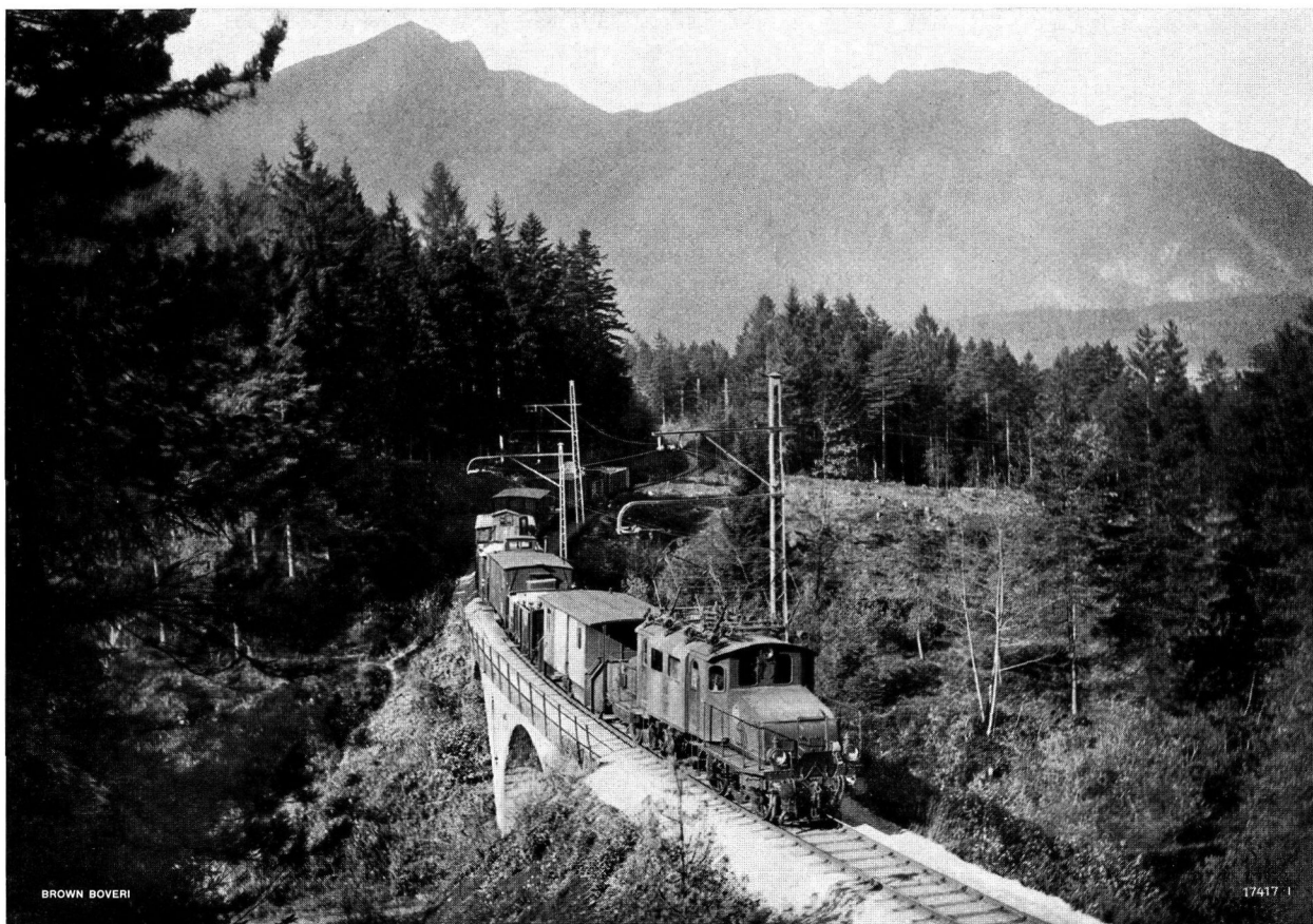
Train of the German State Railway on Freilassing-Berchtesgaden section drawn by B-B locomotive built by Brown, Boveri & Co.
