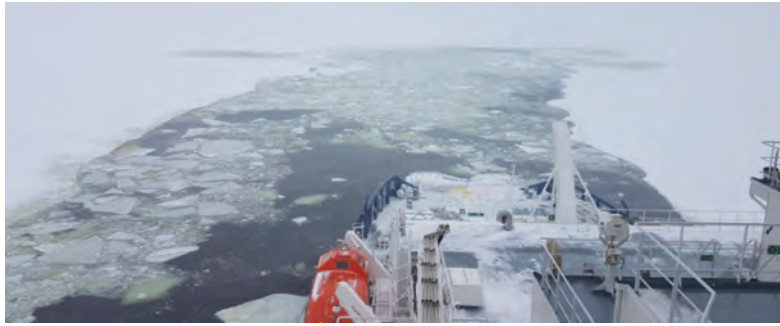
Figure 6: Oblique test widening the ice channel, and thruster orientation
