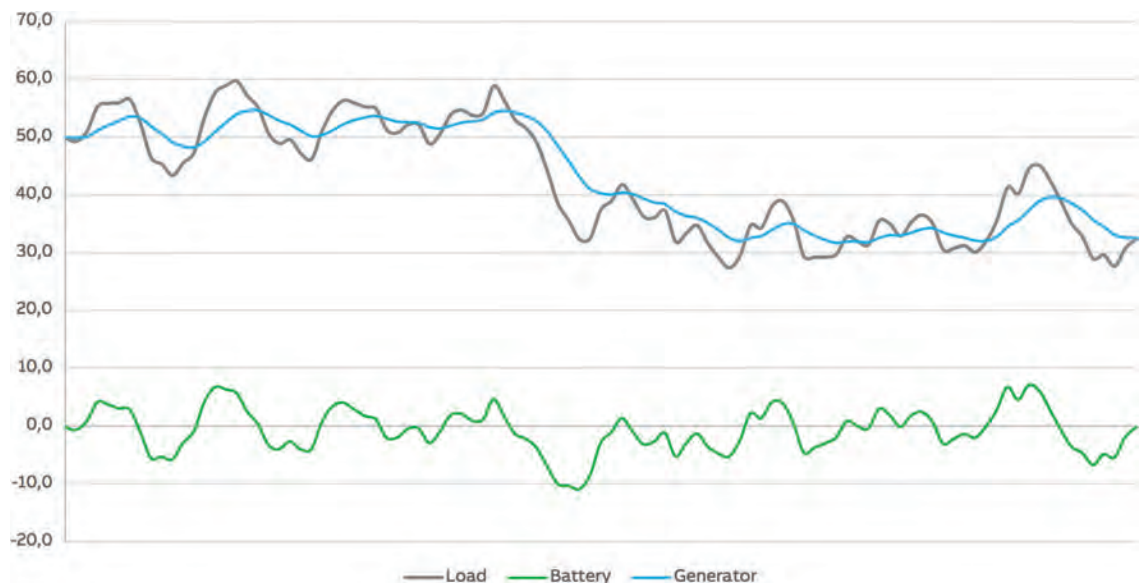
Figure 1: A battery can take the rapid variations and let the engines deliver the mean load on the power plant
