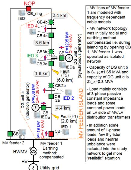
Figure 5. Studied MV network used in PSCAD simulations.
