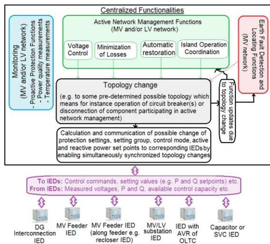
**Figure 1.** An example of some possible centralized functionalities at HV/MV and MV/LV substations.
