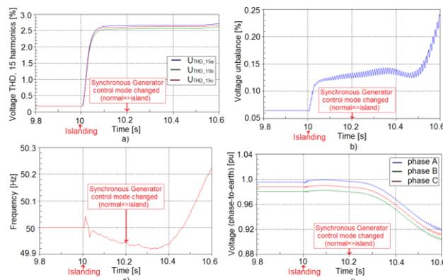
Figure 6. Simulation results from a) voltage THD, b) voltage unbalance, c) frequency and d) voltage behavior after islanding at t=10.0 s with study case shown in Fig. 5.
