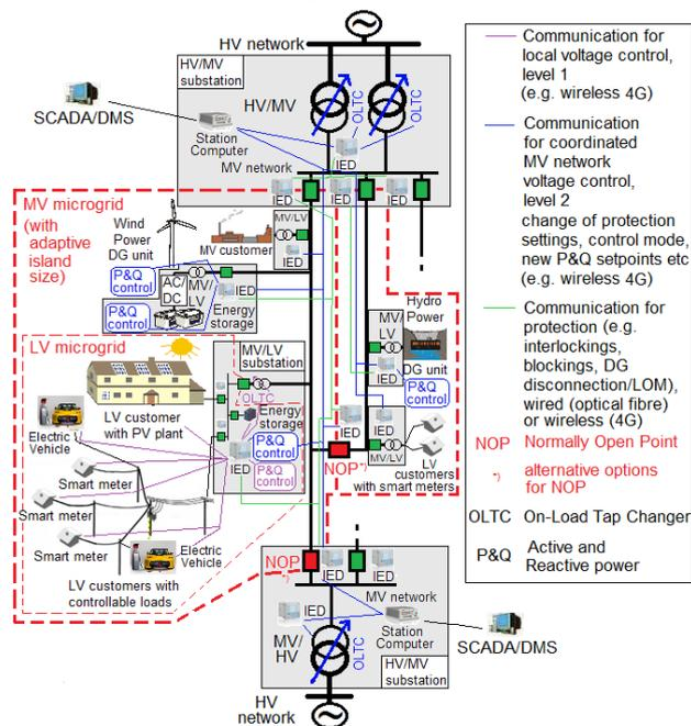
**Figure 2.** Smart Grid compatible IEDs with appropriate communication capabilities and new functionalities will play key role in enabling future active network management and protection concepts.
