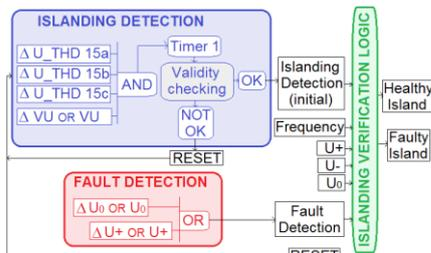
Figure 4. Basic principle of the proposed multi-criteria-based algorithm for islanding detection in distribution networks.
