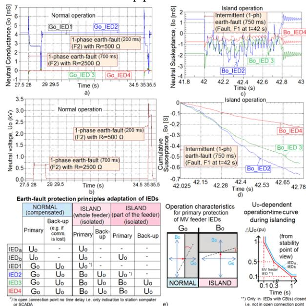
Figure 7. Simulation results about earth-fault protection measurements in a-d) and in e) some example principles/characteristics for earth-fault protection adaptation of IEDs (Fig. 5).
