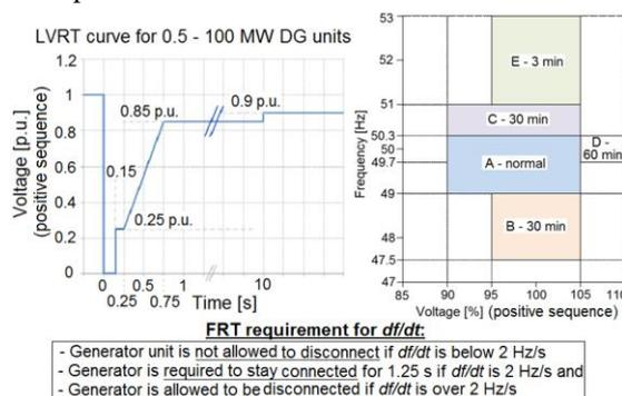
Figure 3. FRT requirements in Finland for 0.5 – 100 MW generator units regarding to voltage, frequency and  $df/dt$  deviations. [2]
