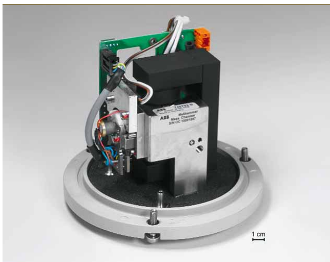
4 A conventional paramagnetic oxygen sensor: parts are assembled manually
