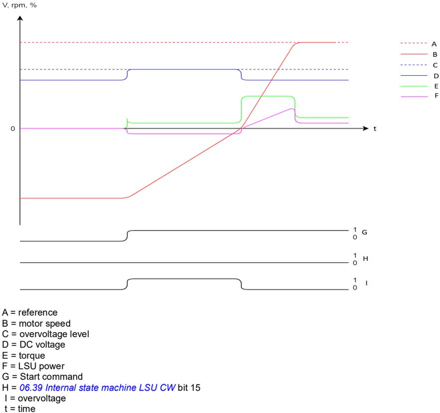
As INU activates the Overvoltage control, it will lower the torque to keep DC voltage at the overvoltage level until the motor speed has reached the zero speed region. If there is a lot of inertia, this can significantly extend the time it takes to reach the requested reference speed
