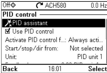
The **PID** submenu contains settings and actual values for the process PID controller. PID is only used in remote control.
