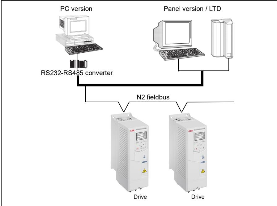
On the N2 fieldbus each drive can be accessed by the full complement of Metasys FMS features, including change-of-state (COS) monitoring, alarm notification, scheduling, trend, and totalization.
