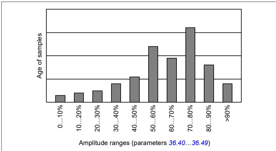
Amplitude logger 1 is fixed to monitor motor current, and cannot be reset. With amplitude logger 1, 100% corresponds to the maximum output current of the drive ( $I_{max}$ ), which is listed in the *Hardware manual* of the drive. The measured current is logged continuously. The distribution of samples is shown by parameters [36.20...36.29](#).
