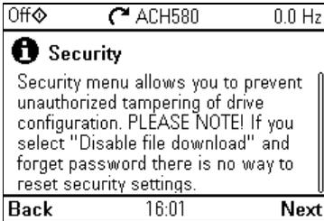
The **Security** submenu is a protected menu that you can open with the user pass code. The menu lets you prevent actions and functionalities with the user lock. You can also change the user lock pass code.
