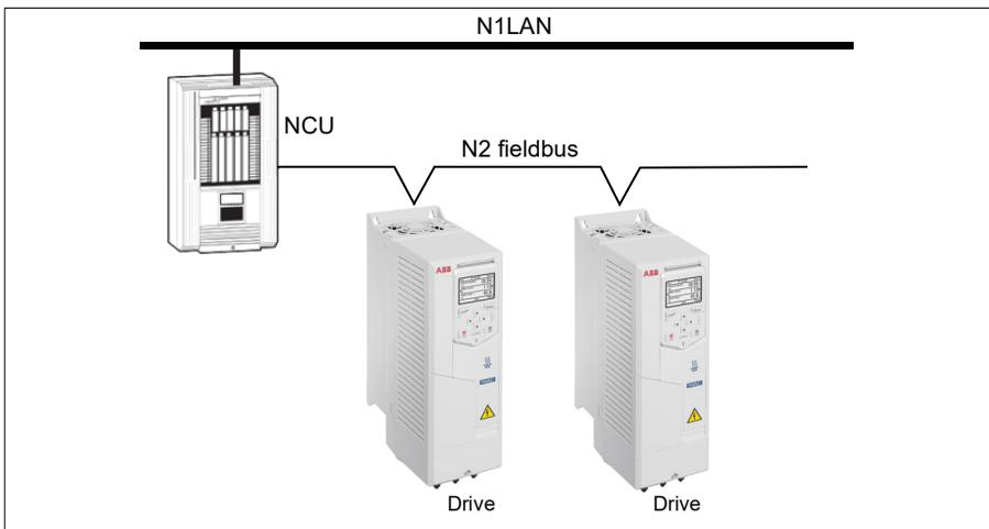
The following diagram shows the drive's integration to the Johnson Controls Metasys Companion system.
