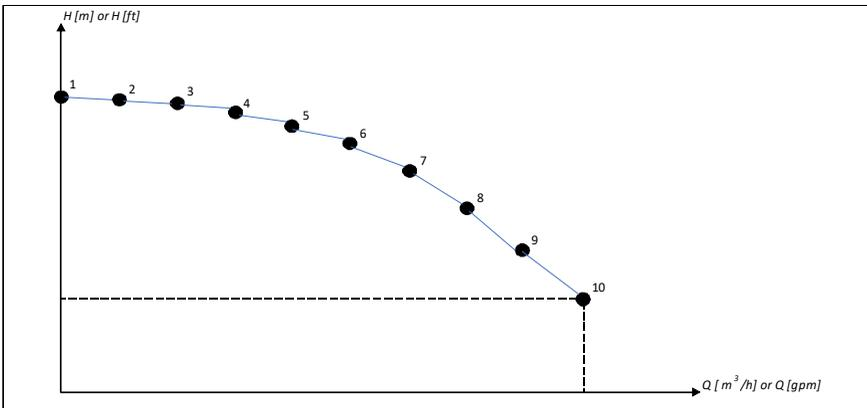
The figure below shows the PQ performance curve of the pump for the flow calculation function.
