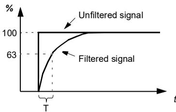
$O = I \times (1 - e^{-t/T})$ <p>I = filter input (step)<br/>O = filter output<br/>t = time<br/>T = filter time constant</p> <p><b>Note:</b> The signal is also filtered due to the signal interface hardware (approximately 0.25 ms time constant). This cannot be changed by any parameter.</p> | 0.100 s       |
