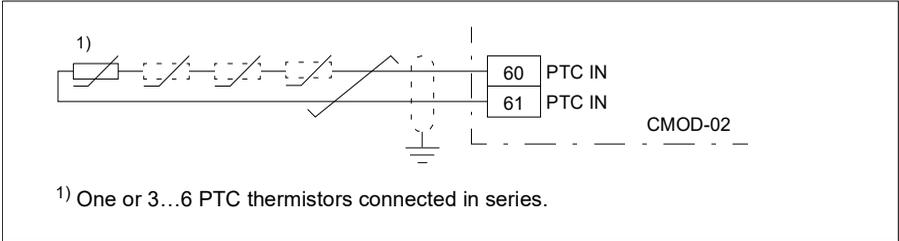
The resistance of the PTC sensor increases when its temperature rises. The increasing resistance of the sensor decreases the voltage at the input, and eventually its state switches from 1 to 0, indicating overtemperature.
