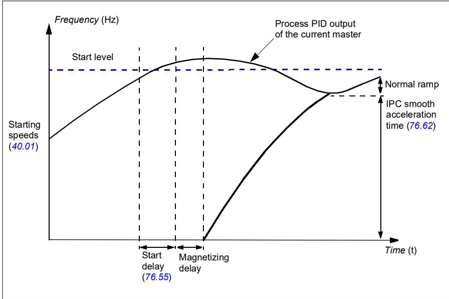
The timing diagram of smooth pump transitions shows the pump starting steps. In this case, the process PID output of the current master has exceeded the start level (76.30...76.32).
