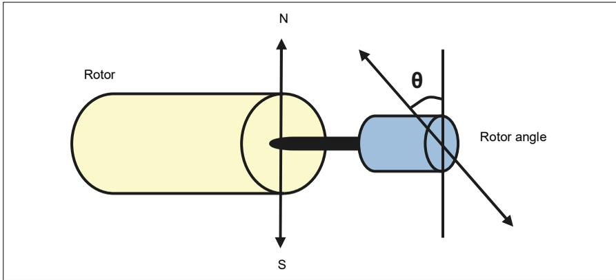
The autophasing routine is performed with permanent magnet synchronous motors to determine the rotor angle at every start.
