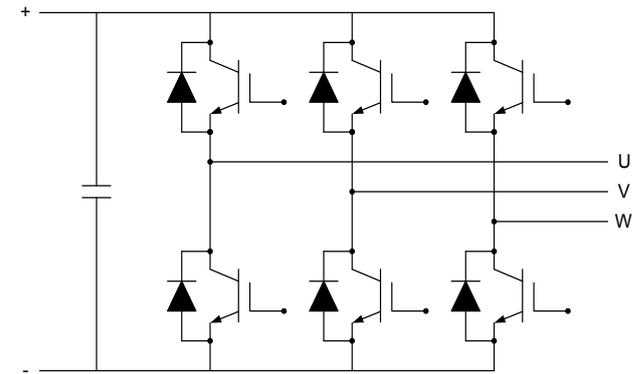
Fig. 4: 2-level voltage source inverter with IGBTs
