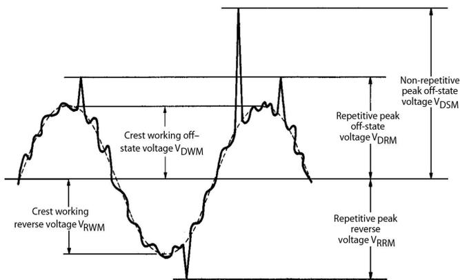
Fig. 1: Definition of repetitive, non-repetitive and normal operating voltages
