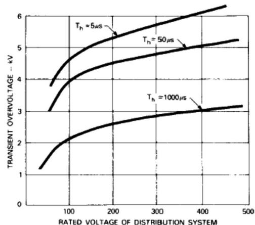
Fig. 3b: Surge amplitudes as a function of nominal line voltage and pulse-width
