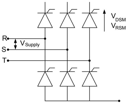
Fig. 2: Voltage definitions based on the example of a three-phase controlled rectifier
