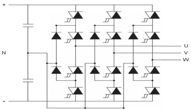
Fig. 5: 3-level Voltage Source Inverter with reverse conducting IGBTs
