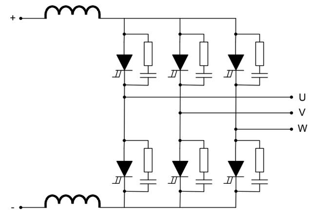
Fig. 6: Current Source Inverter with reverse blocking IGBTs
