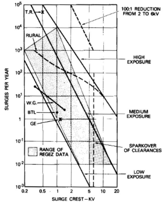
Fig. 3a: Statistical distribution of transients in LV networks
