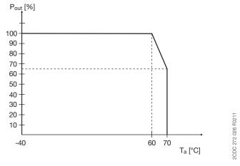
Characteristic curve of temperature at rated load
