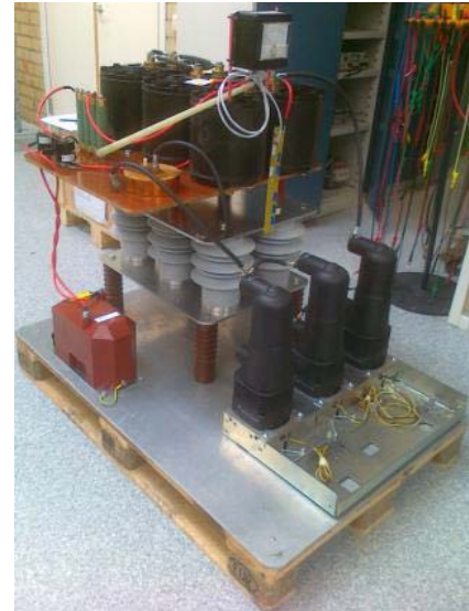
Fig. 6. Vacuum DC circuit breaker with current injection.
