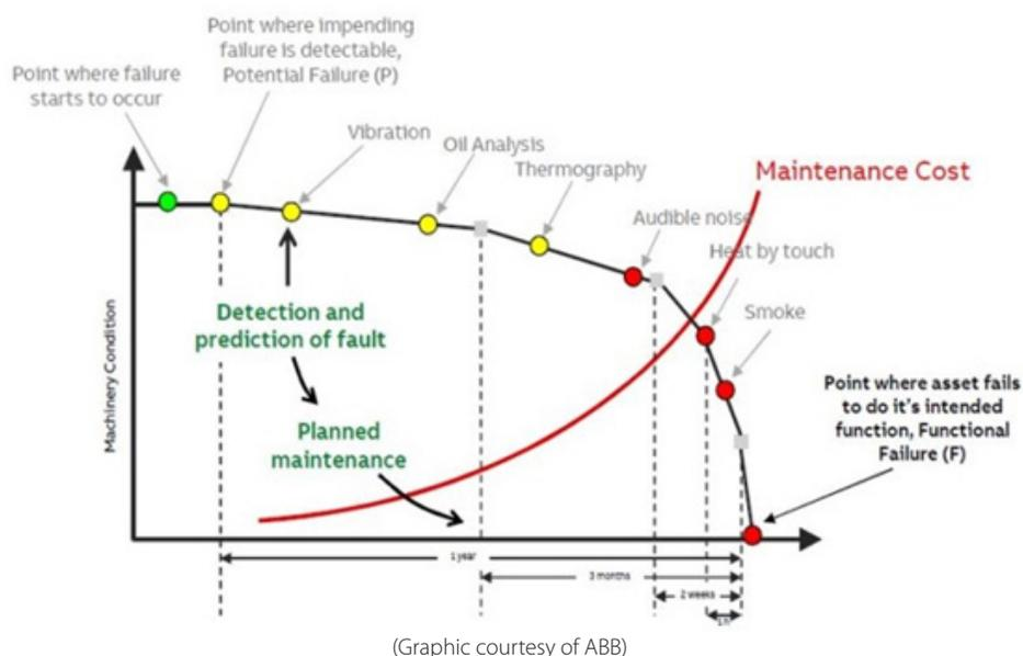
**Figure 2.** Building on a known progression of equipment deterioration, predictive maintenance can alert maintenance workers before declining operation becomes an emergency — regardless of whether that decline is typical, accelerated, or extended. This helps in preventing unexpected downtime and in optimizing scheduled maintenance and maintenance costs vs. emergency repair or replacement.
