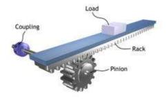
Figure 45 Rack and pinion mechanics
