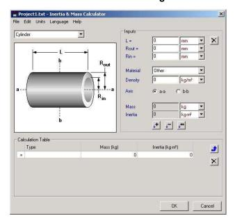
Figure 50 Inertia and mass calculator
