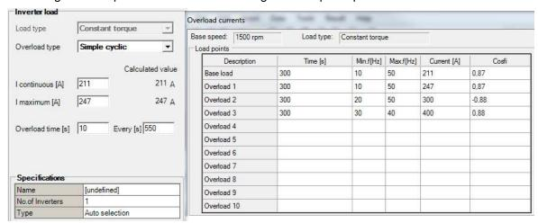
Figure 8: Simple load data for inverter with motor and multiform overload currents given by user without motor.
