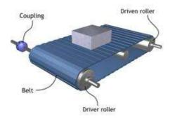
Figure 41 Conveyor mechanics
