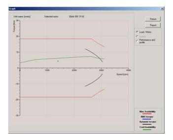
Figure 59 Motor Graph display for Induction Motor
