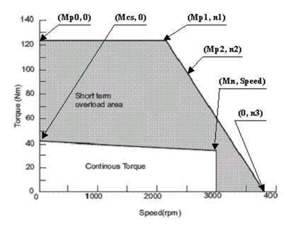
Figure 31 The definition of loadability curve
