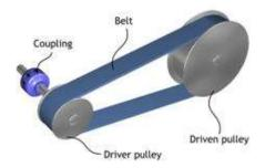
Figure 34 Belt and pulley
