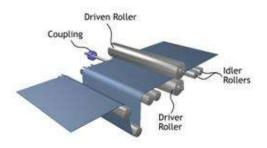
Figure 43 Feedroll mechanics
