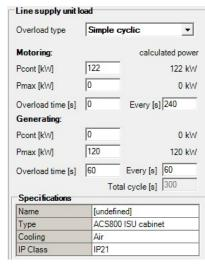
Figure 9: Line supply unit input data and specifications
