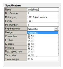
Figure 14: Drop-down list of field weakening frequency
