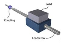
Figure 44 Lead screw mechanics
