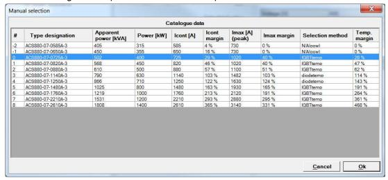
Figure 20: Manual selection view for drive shows the alternative selections. The view is available for motors, drives/inverters and supply units.
