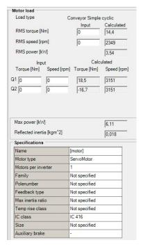
Figure 30 Motor load input data
