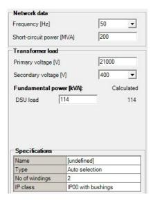
Figure 5: Network/mains data and Transformer load definition
