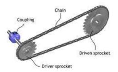
Figure 35 Chain and sprocket
