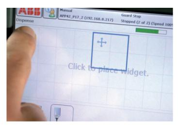
The widget area in Production Screen is a 10 x 4 grid of cells made up of  $60 \times 60$  pixels. ScreenMaker can be used to create widgets that are multiples of  $60 \times 60$  pixels, with a maximum size of  $600 \times 240$  pixels.
