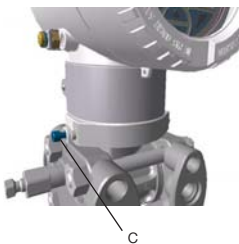
Figure 54: Tang screw removing from the housing
