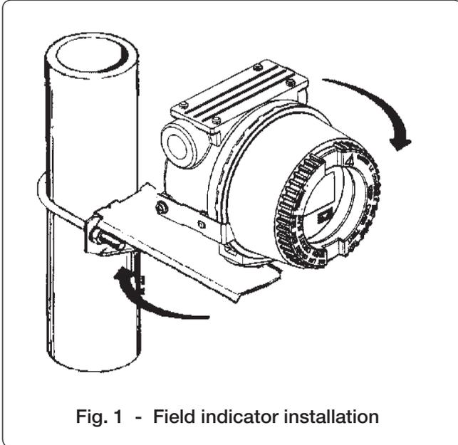
Fig. 1 - Field indicator installation
