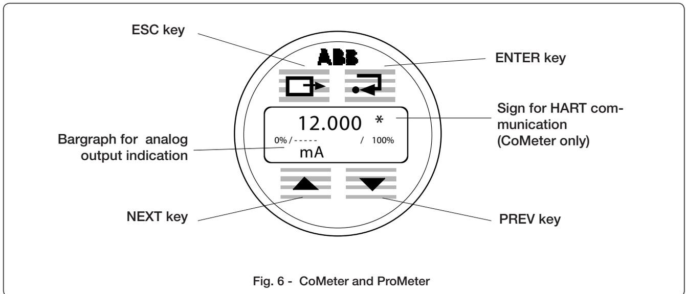
Fig. 6 - CoMeter and ProMeter
