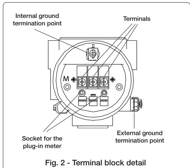
Fig. 2 - Terminal block detail
