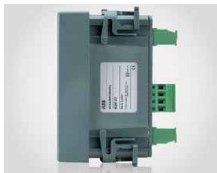
The reduced depth of only 57 mm inside the panel makes the analyser ideal for installation even in switchboard with reduced space. At only 96 mm x 96 mm x 77 mm it still contains everything necessary to measure power quality parameters in real time.
