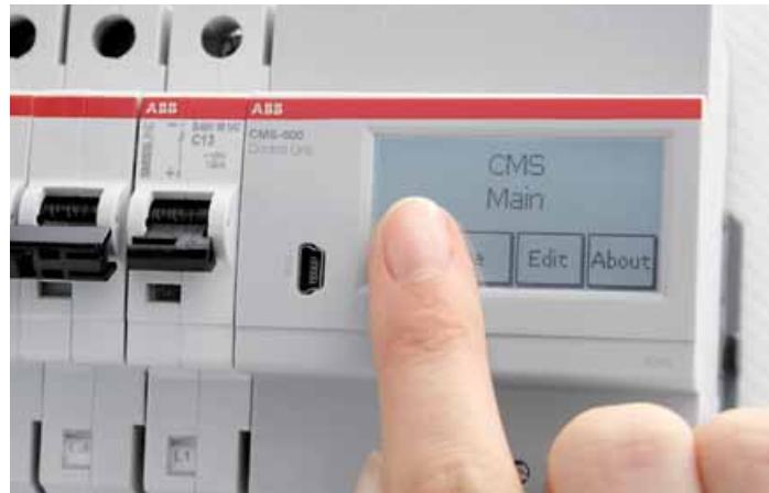
The CMS is a multichannel current measurement system for branch monitoring of alternating (AC) and direct (DC) currents up to 160 A. Various sensor types allow the mounting in every installation environment. Measuring currents within power distribution units (PDUs), very close to the electrical loads, increases the efficiency and availability of every installation.
