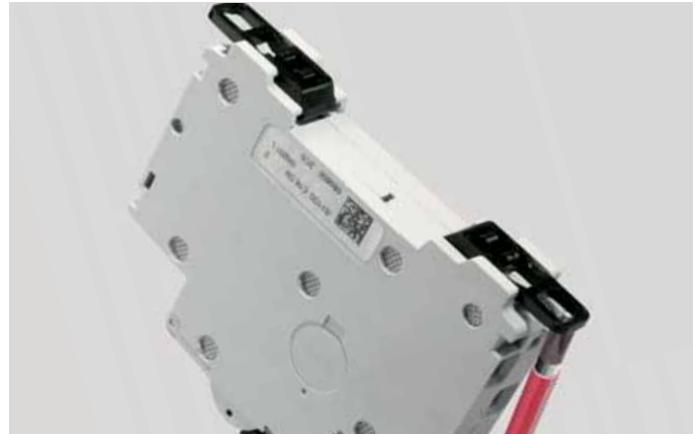
Two bistable fixing devices for maximum ease of use: due to larger size of the DIN rail fixing system, made with 2 bistable fixing devices, the same screwdriver used for tightening the terminals can also be used for assembling and disassembling the device.
