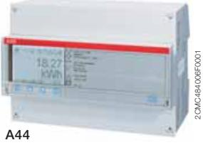
Transformer CTVT connected electricity meter up to 6 A. Verified and approved according to MID. IEC approval. 2- and 3-element metering. Instrument values. Alarm function. Communication - Infrared (M-Bus). Optional - Communication with M-Bus, RS-485 Modbus, RS-485 EQ bus.
