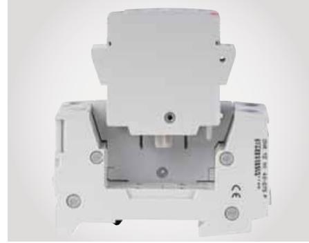
The pluggable feature of ABB surge protective devices (SPDs) facilitates maintenance. Should one or more worn cartridges need to be replaced, the electrical circuit does not have to be isolated nor do the wires have to be removed.
