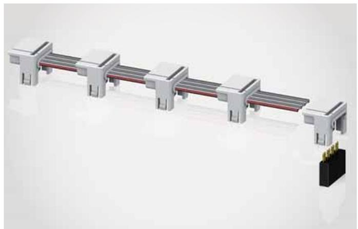
Up to 64 sensors can be connected to each Control Unit. The sensors measure True RMS, AC and DC currents (actual, min/max, hold values) and transmit their measurement data via the flat cable to the Control Unit. The measured values are displayed locally on the Control Unit's touch display and can be queried remotely by an RS485 Modbus connection.
