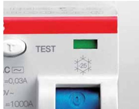
RCCBs F200 can be used in ambient conditions where the temperature of the surrounding atmosphere has values between -25°C (snowflake laser printed on the front of the device) and +55°C.
