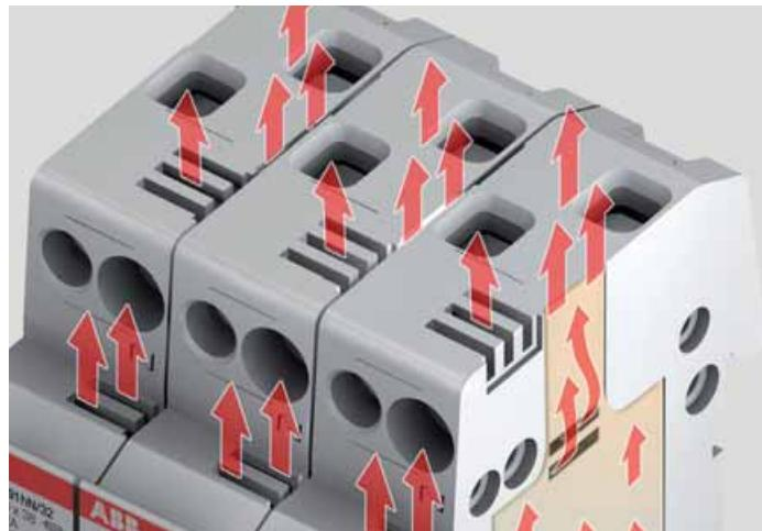
Venting grooves and cooling chambers improve heat dissipation even in multiple-pole configurations. The reduced operating temperature inside fuseholders ensures durability and reliability of the devices over time.
