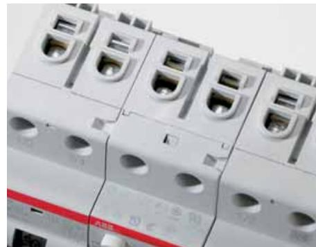
The terminals available on DS201-DS202C make easier the supply operation in parallel with busbars as they are composed by two different seats, a front seat for 25 mm<sup>2</sup> cables and a back seat for 10 mm<sup>2</sup> busbars.
