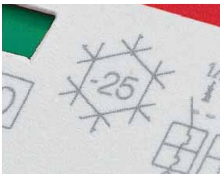
All the devices of the DS201 and DS202C series have been tested in a wide range of temperatures: from -25 °C (as indicated by the snowflake marked on the front side) up to +55 °C.
