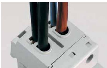
Without busbars two terminal spaces can be used for cables with different cross sections: incoming supply with supplementary terminal up to 50 mm<sup>2</sup> from the front side.
