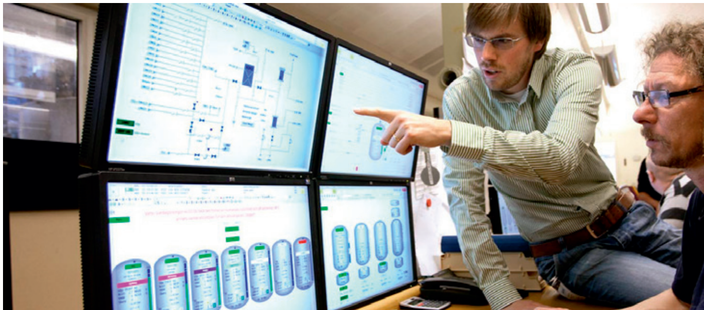
With System 800xA installed in the hydration factory, operator Douglas Ternström avoids much manual reporting and now has full control of what is happening in the process. Magnus Hammar of ABB follows the work closely.
