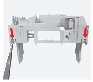
By means of the pliers remove the UVR rod mounted on the breaking part cover.
