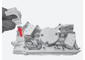
Manually remove the arching chambers.
