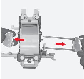
Manually remove the operating mechanism from the central pole.
