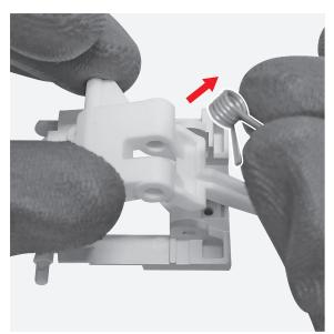
By means of the pliers remove the benzing mounted on the RC group release.
