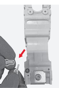
Manually remove the insert and the I3 lever.
