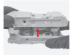
**46** Manually remove the terminal protection.
