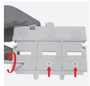
By gravity let the 3 fixed cores separate from the trip unit cover.
