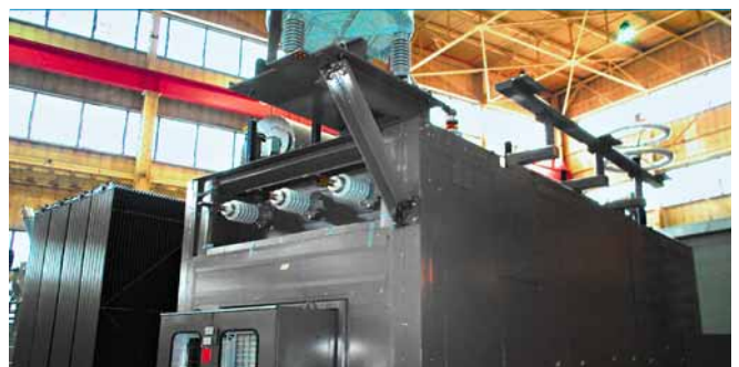
9 Ultra-low noise ConEd transformer with Sound Enclosure
