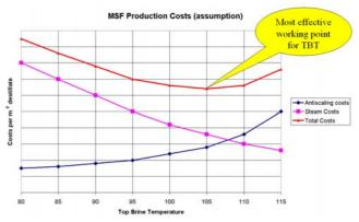
The steam costs per m3 distillate decreases with higher TBT because the Performance Ratio (PR) increases.
