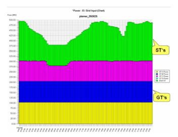
Above graphic shows an example for a pre planned optimized day ahead schedule for the gas and steam turbines created by **PowerFit**. In this example only three of the four GTs are running. The load change over the day is adjusted by the steam turbines.
