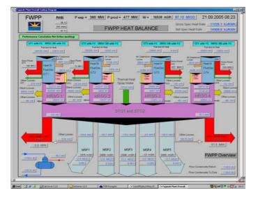
The graphics and the respective trends are used for analysing the performance of the entire plant as well as for individual areas. Comparisons between actual and expected performance in connection with supervisory identifiers makes the analysis simple and effective.
