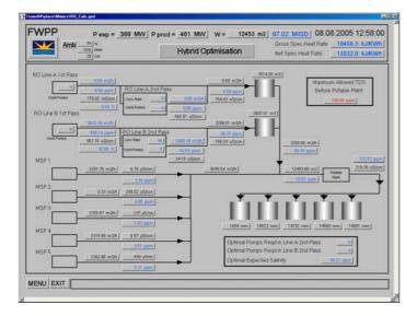
The above graphic is used in Fujairah for Hybrid Optimization. In this production example 2second pass racks can be taken out of service compared to the standard approach by using 1 second pass rack for every 2 first pass racks in operation (1:2 ratio).
