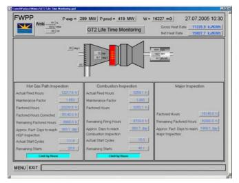
GT and ST lifetime monitoring algorithm give an indication to the current lifetime of the equipment, based on operating hours, start/stop cycles etc. and also information on how much longer the equipment can be run before an inspection is recommended by the equipment manufacturer.
