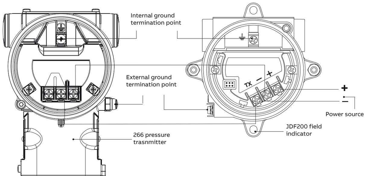
Figure 2 JDF200 Wiring drawings
