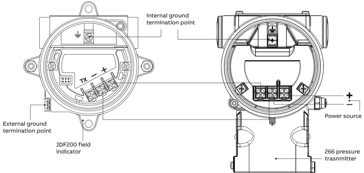
NOTE – This wiring as remote indicator is not applicable for 266 pressure transmitter with surge protection option code S2
