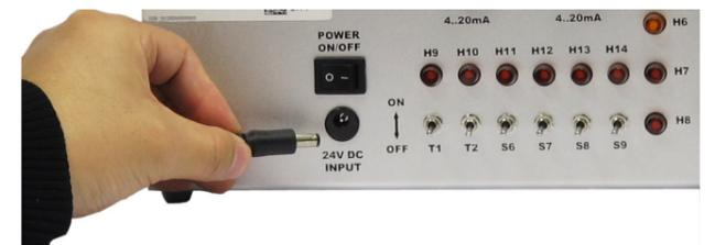
3. *en* Connect the power adaptor to socket 24 V DC INPUT
