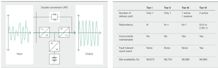
In a Tier IV data center, a "system + system" configuration, namely two separate UPS systems, each with N + 1 redundancy, enables infrastructure work to be undertaken without disrupting the critical load.
