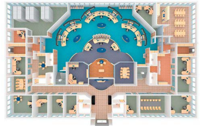
Design for the layout of a control room. Effective facility design puts all the resources, operators, and production management needs within easy reach. Courtesy: ABB
