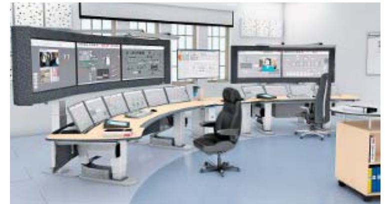
ABB's Extended Operator Workplace. The right combination of equipment and ergonomics creates an environment that lowers stress levels and allows operators to improve situational awareness. Courtesy: ABB
