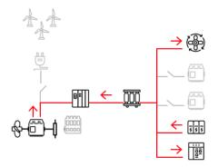
The shaft generator is the vessel's main source of propulsion. This is intended for emergency or short-term use: it enables the vessel to return safely to port when the main engine is out of operation. The PTH function provides redundancy and safety. The shaft has to be fitted with a clutch to enable disconnection of the main engine when PTH mode is activated. In PTH mode the VSD controls the shaft generator / motor with input from the propulsion system.
