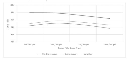
PM technology is more efficient than synchronous and induction technology across the entire speed range (theoretical comparison).
