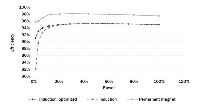
Permanent magnet generators are more efficient than induction generators at all power levels.
