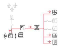
PTO or generator mode uses the energy efficient main engine to produce power. The generator and VSD can be supplied to operate in:
