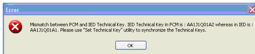
Figure 30: Error message due to mismatch between PCM600 and IED technical key
