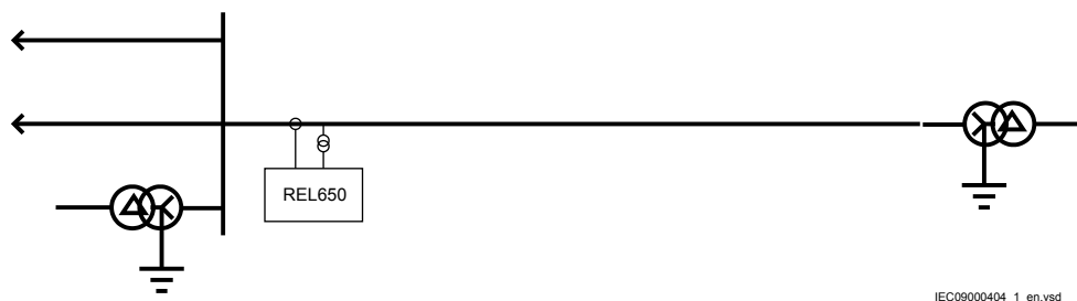
Figure 7: Two-ended over-head line with transformer in a solidly earthed network
