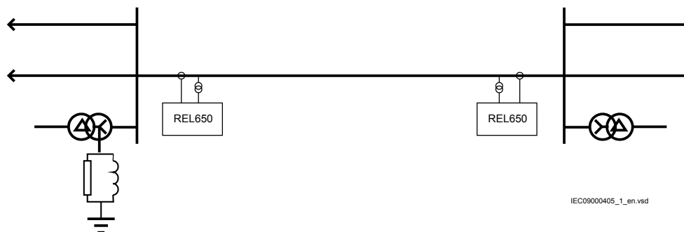
Figure 8: Two-ended over-head line in a high-impedance earthed network
