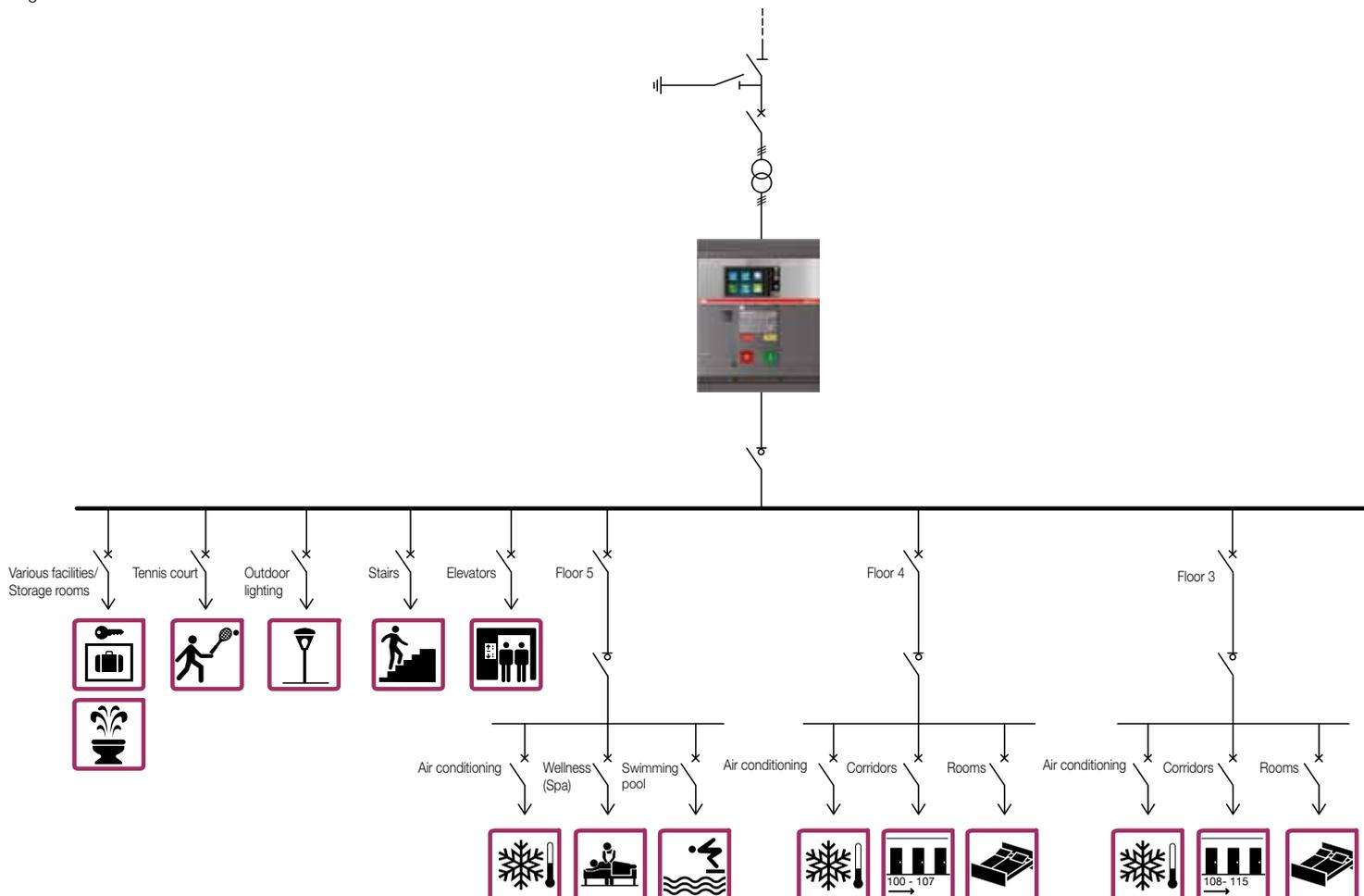
Therefore, in order to reduce the maximum contractual power agreed upon with the DSO, through *Ekip Power Controller* function the aim is to decrease the maximum power absorption at 500 kW.
