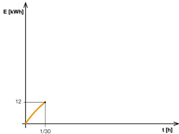
As time passes, the point describing the state of the system moves towards higher values of  $t$ . Energy  $E$  is increasing or however it can remain constant if the energy consumption is null. Then, the total energy absorption is described by the curve of Figure 4.
