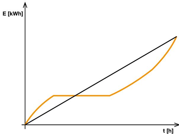
Since *Ekip Power Controller* is aimed at keeping the total value of energy in the reference period below the set limit, the software examines the trend of the curve up to the current moment and evaluates the energy consumption at the end of the period, verifying that the ratio between such consumption and the predefined period does not exceed the contractual power limit. If this limit is exceeded, the disconnection of one or more loads is commanded.
