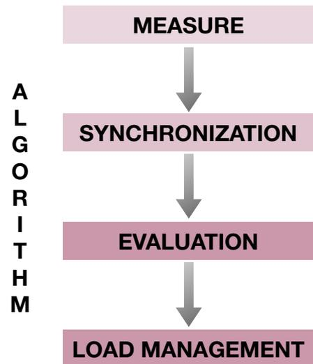
1. *Measure*: it measures the total power flow through the circuit breaker SACE Emax 2 which implements the function. Afterwards, this value is integrated to obtain the total energy. When each reference time interval has elapsed, the energy is set to zero. In such way, the evaluation modulus of the algorithm has always at its disposal the value of the energy measured in the current interval of time.
