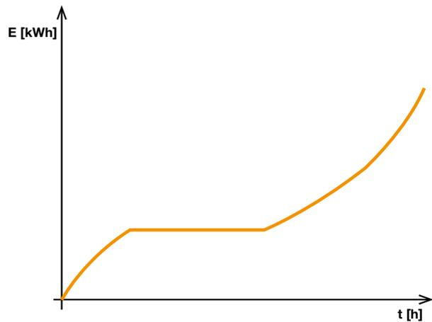
The same total value of energy can be obtained with very different trends; if, for example, the power value is constant, a line going through the origin of the axes is obtained. But the same value can be obtained also with a low con-
