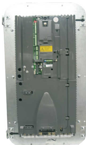
ACS550 R5 - R6 Frame with sealing spacers and flange plates in place.
