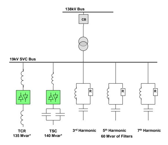
TCR: Thyristor Controlled Reactor TSC: Thyristor Switched Capacitor
