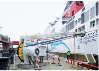
Connecting Stena Hollandica to the local grid
