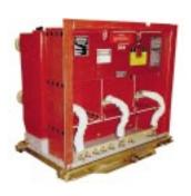
A "G&T device" is a drawout assembly compatible with circuit breaker compartments. The G&T provides a means to select and test primary circuits in a controlled manner, and then to connect deenergized primary circuits to the switchgear ground bus to support maintenance activity. Refer to drawing on page 52 in the Reference Section.
