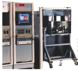
ADVAC circuit breakers are automatically tested and cycled 300 operations prior to shipment.
