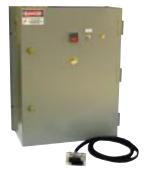
A "test cabinet" is a wall-mounted control cabinet connected to a separate power source and containing switches to open and close a breaker. The test cabinet has a female connector and an umbilical cord (stored inside the cabinet) for connection to the breaker, and serves as an aid to breaker inspection and maintenance in switchgear aisles or work areas.
