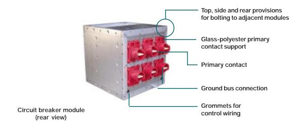
Each module has bolt provisions for connection to upper or lower modules in the same vertical section, connection to modules in adjacent vertical sections, and attachment of primary bus barriers and rear cable compartments fabricated by the switchgear assembler.
