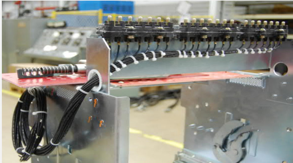
Example of AK25 Secondary Disconnects (Images)
