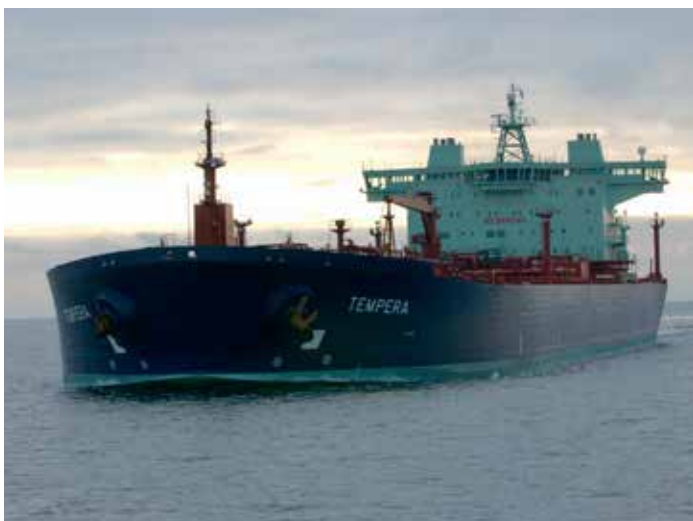
Crude oil tanker Tempera with 16MW Azipod VI
