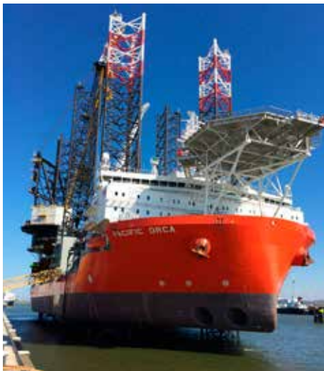
Wind Turbine Installation vessels Pacific Orca has 4 pcs 3.4MW Azipod CO thrusters
