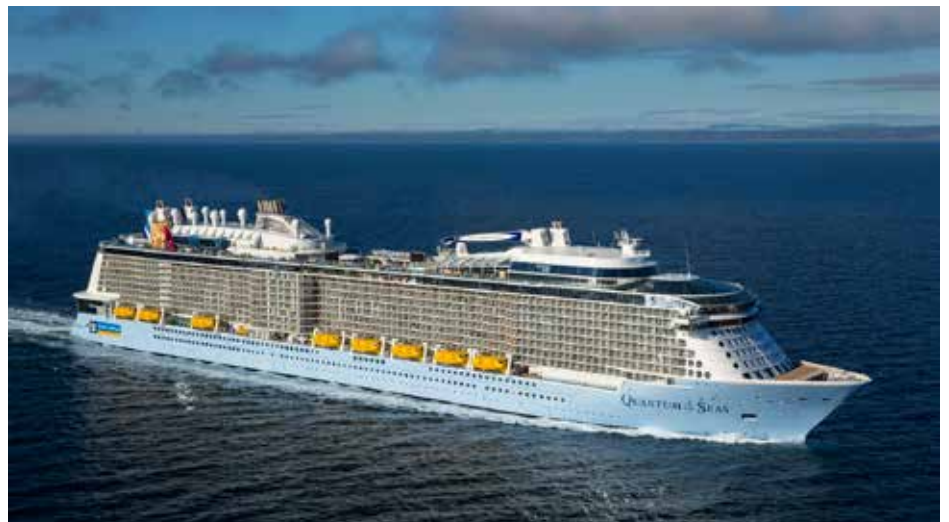
Quantum of the Seas has 2 pcs 20.5MW Azipod XO units
