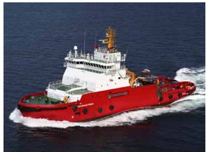
Icebreaking tug Polar Pevek with 2 pcs 5MW Azipod VI propulsion units
