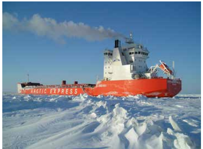
Arctic container vessel Norilsk Nickel with single 13MW Azipod VI propulsion
