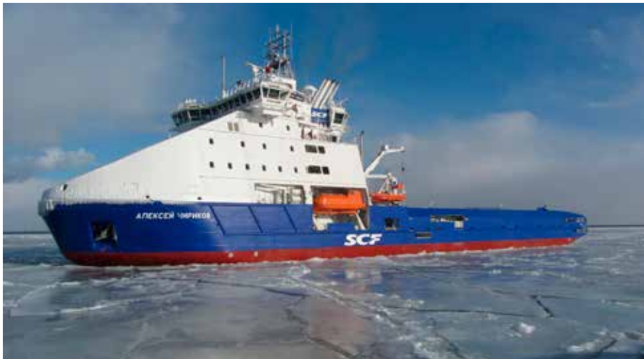
Icebreaker supply vessel Aleksey Chirikov is equipped with 2 pcs 6.5MW Azipod VI propulsion units
