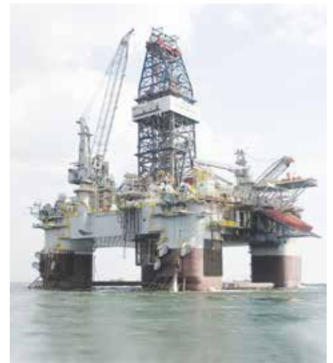
Semi-submersible drilling rigs Development Driller I and II have both 8 pcs 3.2MW Azipod CZ thrusters
