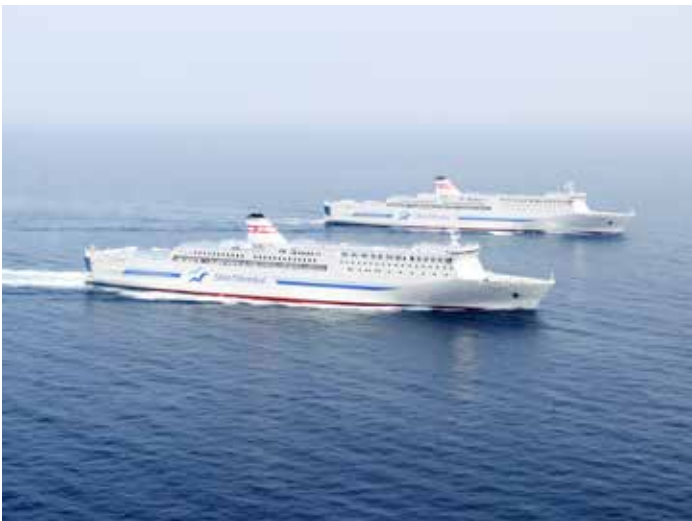
High speed ferries Akashia and Hamanasu have CRP Azipod propulsion with 17.6MW Azipod V propulsion unit and 24.4MW diesel driven propeller
