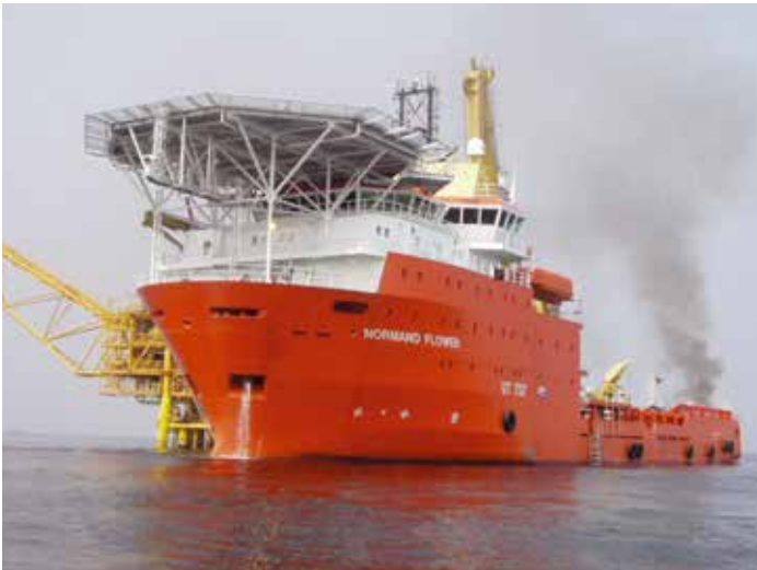
Offshore supply vessel Normand Flower is equipped with 2 pcs 2.3MW Azipod CO units
