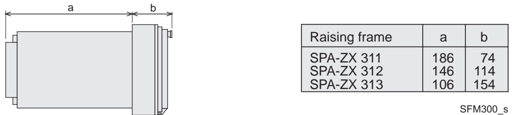
Fig. 3 Semi-flush mounting relay case (dimensions in mm)
